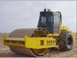
Intelligent compaction rollers are equipped with a speed sensor, an accelerometer to measure drum vibration, and a processor that analyzes this data and sends it to a unit that displays a color-coded map of stiffness in the area being compacted.
