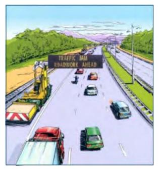
Figure 2. Portable sign gantries in the Netherlands (Steinke et al. 2000)
