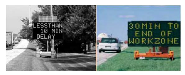
Figure 3. Examples of delay and travel time estimation system displays (FHWA 2001b)
