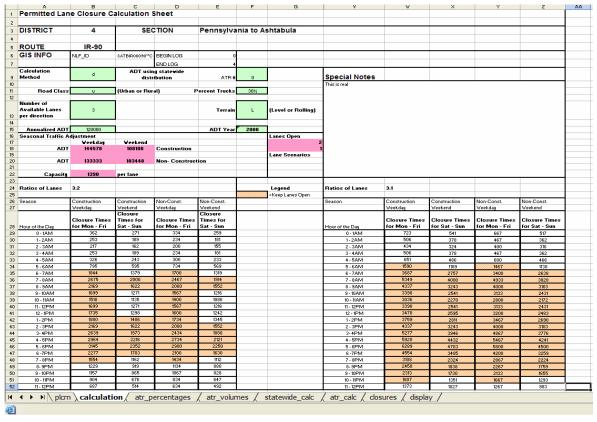
Figure 9. ODOT permitted lane closure calculation spreadsheet (ODOT 2006)
