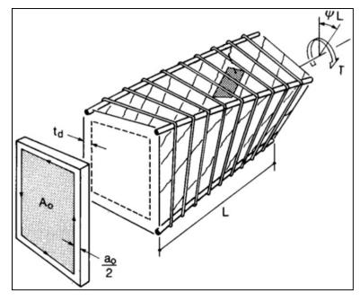
Figure 2.16: Post-Cracking Hollow Tube Analogy (Collins & Mitchell, 1991)
