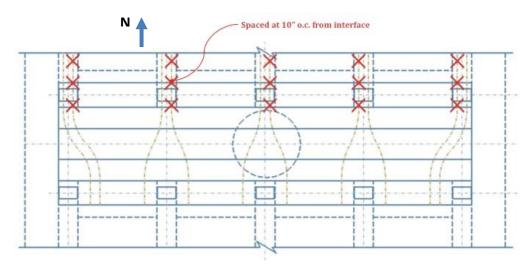
Figure 6.52: Unstressed strand strain gauge locations
