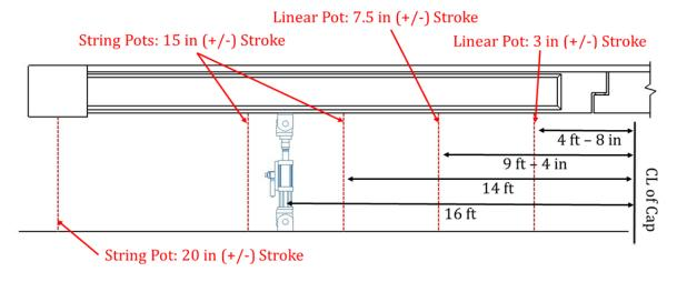
Figure 5.39: Phase 2 Vertical Girder Displacement Device Locations
