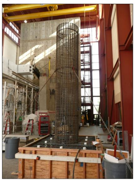
Figure 5.2: Completed Column and Footing Cage
