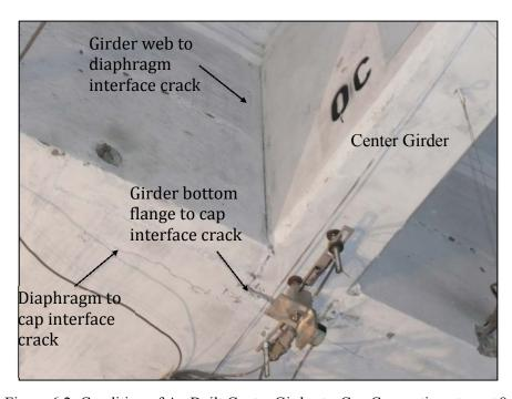
Figure 6.2: Condition of As-Built Center Girder-to-Cap Connection at  $\mu_{\Delta}$ =+8
