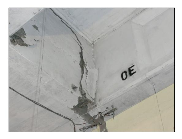
Figure 6.35: Damage to As-built Connection Exterior Girder at +2 in. Displacement
