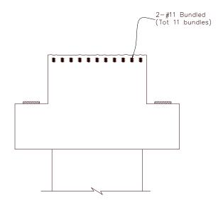
Figure B.4. Cap Beam Top Flexural Reinforcement
