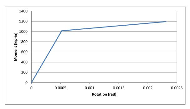
Figure 4.24: Improved Connection Predicted Moment vs. Rotation Response
