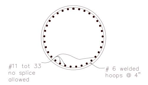
Figure B.2. Column Reinforcement Layout
