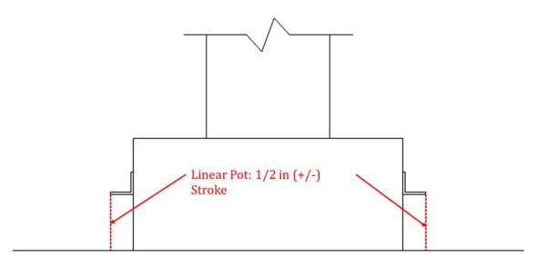
Figure 5.47: Footing Uplift Device Locations
