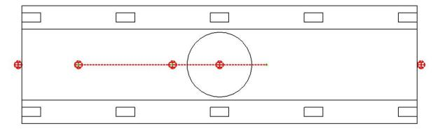
Figure 5.42: Plan View of Cap Beam Twist and Dilation Instrumentation Scheme
