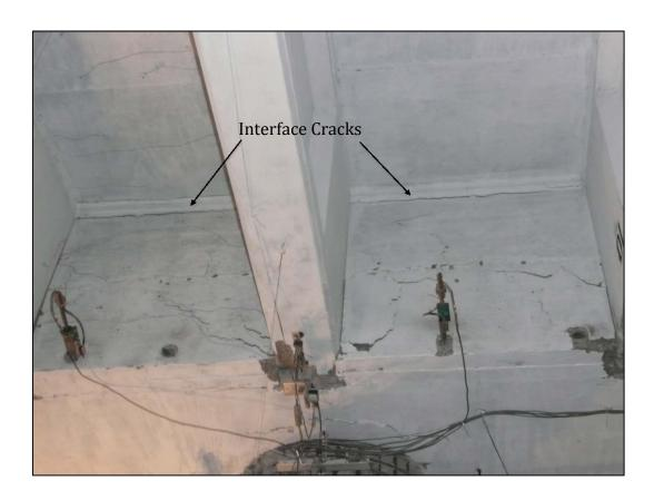
Figure 6.34: Deck-to-Diaphragm Interface Cracking at +1 in. Displacement
