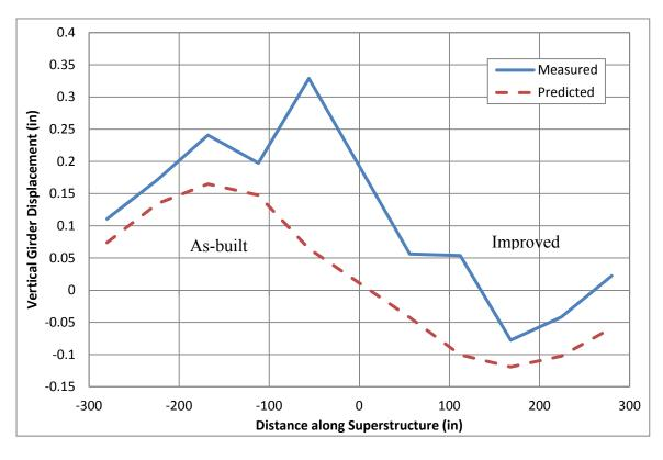
Figure 6.10: Center Girder Vertical Displacements at  $\mu_{\Delta}$  = -8
