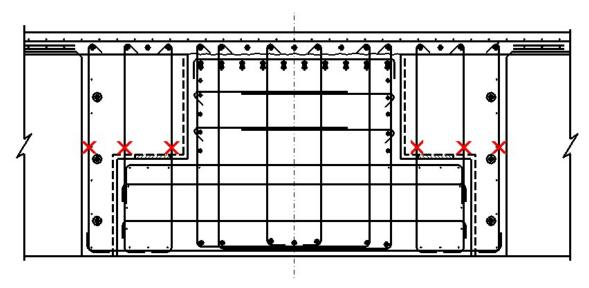
Figure 5.26: Cap Beam Outer Stirrup Strain Gauge Locations
