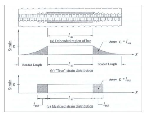
Figure 2.18: Bond-Slip Unbonded Length (Raynor et. al., 2002)
