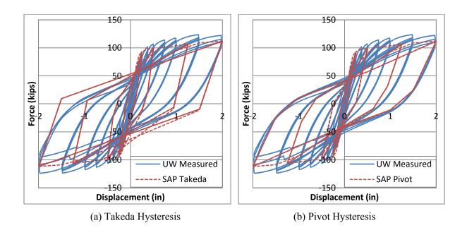
Figure 4.15: Force-Displacement Hysteresis Comparison
