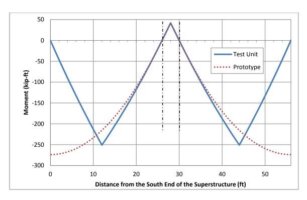
Figure 5.53: Stage 1 Prototype-to-Test Unit Moment Profile Comparison along the Length of the Superstructure after Applying Stage 1 Hold-Down Force
