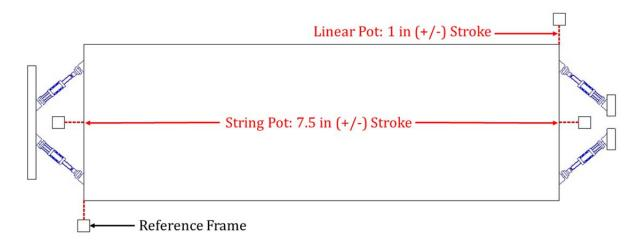
Figure 5.35: Location of Deck Displacement Devices
