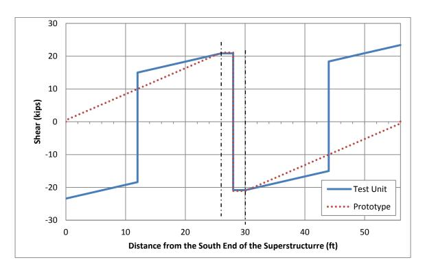
Figure 5.54: Stage 1 Prototype-to-Test Unit Shear Profile Comparison along the Length of the Superstructure after Applying Stage 1 Hold-Down Force
