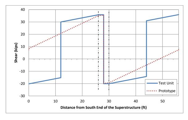
Figure 5.58. Final Prototype-to-Test Unit Shear Profile Comparison along the Length of the Superstructure after Applying Hold-Down Forces and Seismic Effects
