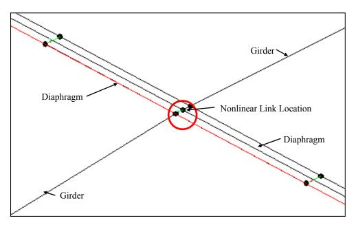
Figure 4.20: Grillage Model Girder-to-Cap Nonlinear Link Location
