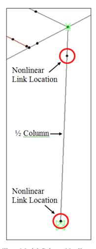
Figure 4.12: Grillage Model Column Nonlinear Link Locations
