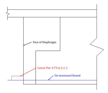
Figure 5.45: Strand Slip Device Location
