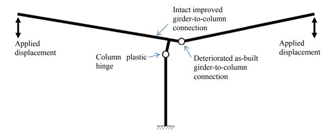
Figure 6.40: Rotation of girders about as-built connection
