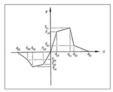
Figure 2.13: Typical Strength Envelope (Dowell et. al., 1998)
