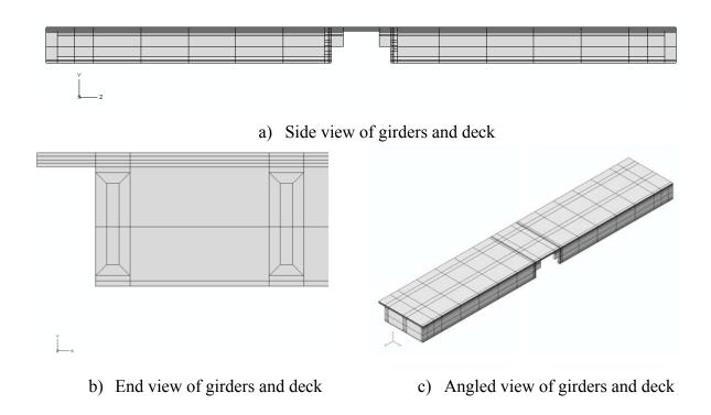
Figure 4.7. Views of the modeled girders and slab of model
