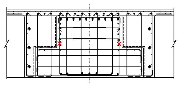
Figure 5.24: Cap Beam Inner Stirrup Strain Gauge Locations
