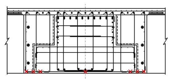
Figure 5.22: Cap-to-Diaphragm Hooked Reinforcement Strain Gauge Layout
