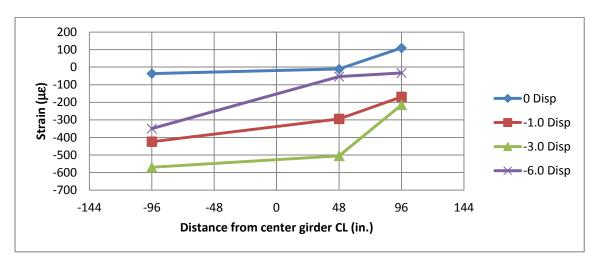
Figure 6.53: Transverse strain profiles from unstressed strands in improved connection (from gauges located 10" north of interface)
