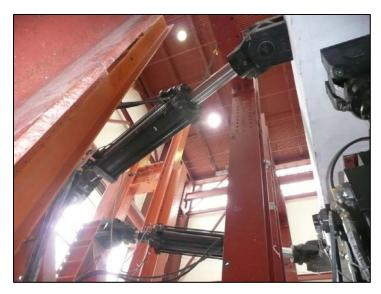
Figure 5.48: Horizontal Actuator Configuration used during Phase 1 Testing at Each End of the Test Unit
