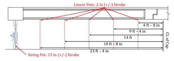
Figure 5.37: Phase 1 Vertical Girder Displacement Device Locations
