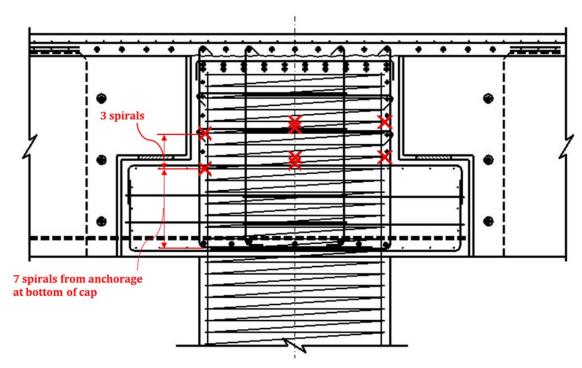
Figure 5.16: Column-to-Cap Beam Spiral Instrumentation within the Joint
