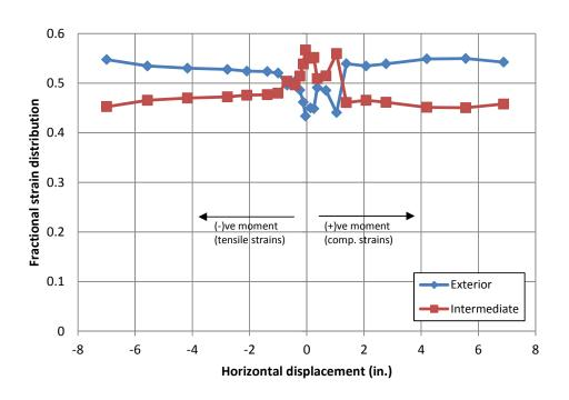
Figure 6.27: Contribution of Moment Resistance by Girders on the As-built Connection Side 1.5 feet from the Diaphragm Edge
