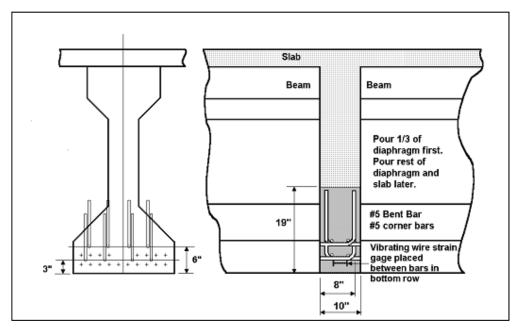
Figure 2.3. NCHRP Bent Bar Specimen (Miller et. al., 2004)
