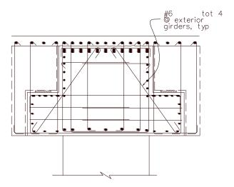
Figure B.14. Corbel diagonal cracking reinforcement
