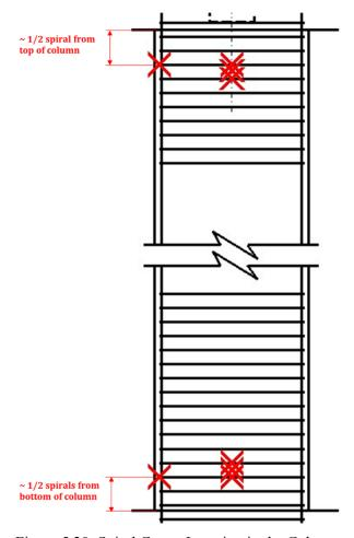
Figure 5.20: Spiral Gauge Location in the Column
