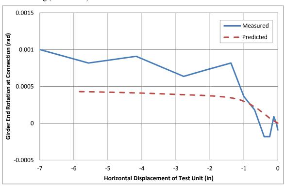
Figure 6.15: Center Girder Improved Connection Girder Rotation/Gap Opening
