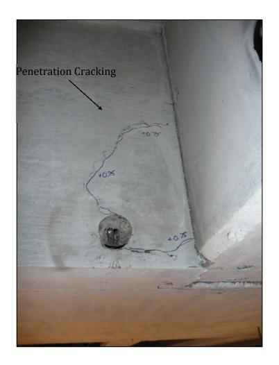
Figure 6.32: Penetration Cracks on the Face of the Diaphragm on the As-built Connection Side at +0.75 in. Displacement (Repeated)
