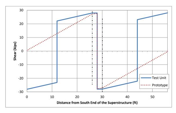
Figure 5.56: Stage 2 Prototype-to-Test Unit Shear Profile Comparison along the Length of the Superstructure after Applying Additional Stage 2 Hold-Down Force
