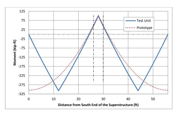
Figure 5.55: Stage 2 Prototype-to-Test Unit Moment Profile Comparison along the Length of the Superstructure after Applying Additional Stage 2 Hold-Down Force
