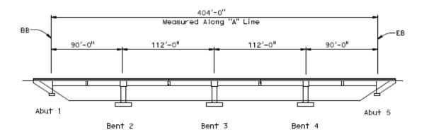
Figure B.1: Prototype Elevation
