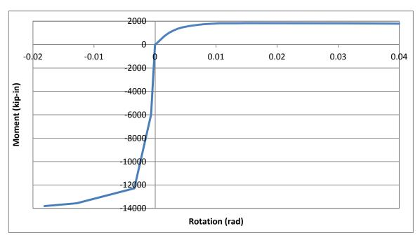
Figure 4.19: Girder-to-Cap Connection Intermediate Girder Moment-Rotation Response
