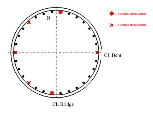
Figure 5.17: Location of Gauged Longitudinal Column Reinforcement
