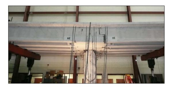
Figure 6.37: Overall Response of Test Unit at +3 in. of Vertical Displacement
