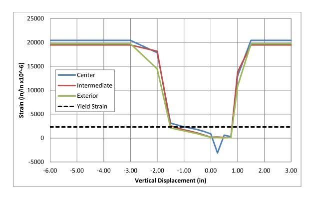
Figure 6.29: Vertical Displacement vs. Deck Reinforcement Strain above the Inverted-T Stem on the Asbuilt Connection Side of the Cap Beam at Each Girder
