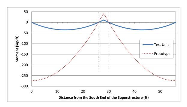
Figure 5.51: Stage 1 Prototype-to-Test Unit Moment Profile Comparison along the Length of the Superstructure without Scaling Compensation
