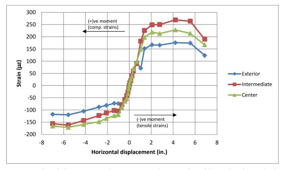
Figure 6.23: Deck Reinforcement Strains on Improved Connection Side 1.5 feet from Diaphragm Edge, above the Exterior, Intermediate, and Center Girders
