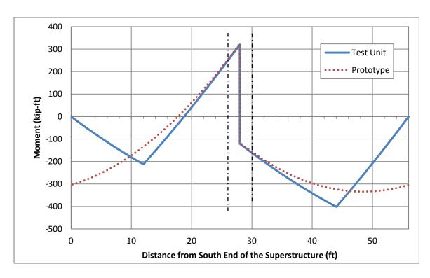
Figure 5.57: Final Prototype-to-Test Unit Moment Profile Comparison along the Length of the Superstructure after Applying Hold-Down Forces and Seismic Effects
