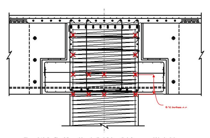
Figure 5.18: Profile of Gauged Longitudinal Column Reinforcement within the Joint
