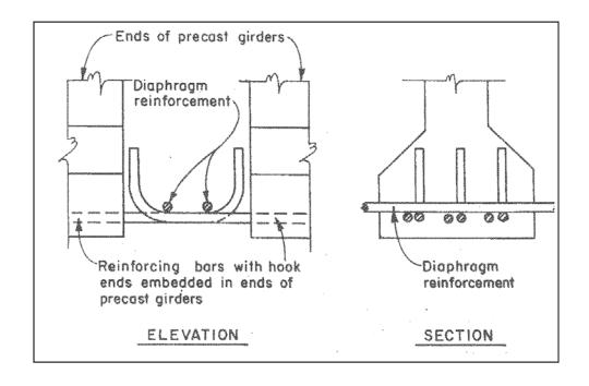
Figure 2.1. Connection Selected for Testing by Freyermuth (1969)
