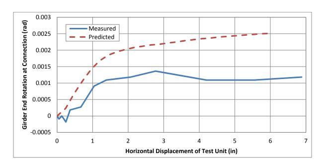
Figure 6.6: Center Girder End Rotation within Girder-to-Cap Connection vs. Horizontal Displacement during Phase 1 Testing
