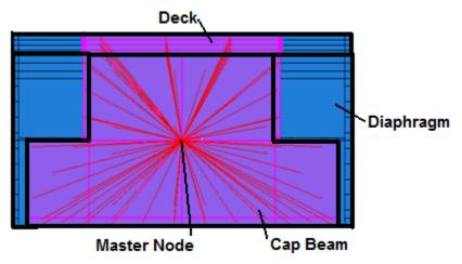
Figure 4.4. Cap Beam pivot constraint achieved through the use of the coupling command
