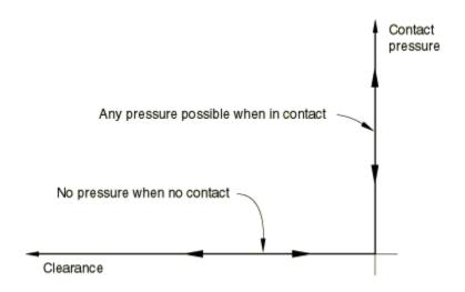
Figure 4.3. "Hard" contact behavior assumed in ABAQUS
