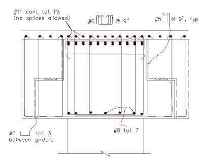
Figure B.7. Cap Beam Reinforcement under Service Load Conditions
