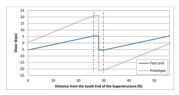
Figure 5.52: Stage 1 Prototype-to-Test Unit Shear Profile Comparison along the Length of the Superstructure without Scaling Compensation
