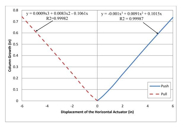
Figure 5.50: Horizontal Actuator Displacement vs. Column Growth
