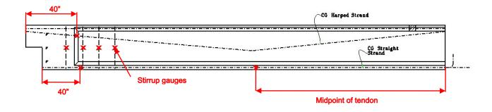
Figure 5.29: Girder Strain Gauge Layout
