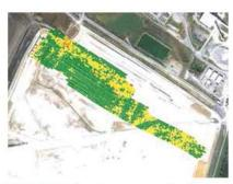
Figure 3.1C data from study on compaction of CCPs showing weak areas.
