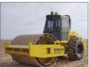
Intelligent compaction rollers are equipped with a speed sensor, an accelerometer to measure drum vibration, and a processor that analyzes this data and sends it to a unit that displays a color-coded map of stiffness in the area being compacted.
