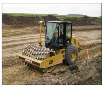
Figure 1. Caterpillar CP563 padfoot roller with MDP\* measurement system on TH 60 project (from
