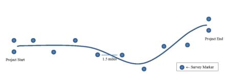
Figure S-xx.5 Schematic of the required Survey Marker configuration.
