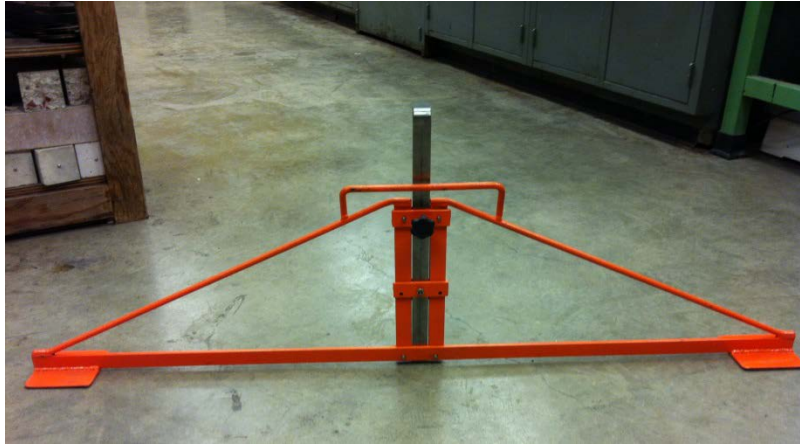
Figure 17. Deflectometer for measuring rutting
