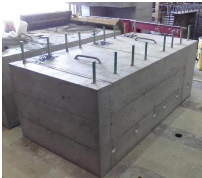
Figure 24. Grouted coupler pile cap
