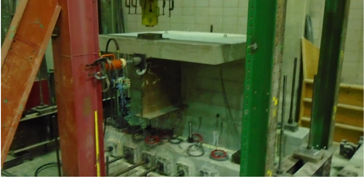
Figure 55. Laboratory loading and horizontal and vertical actuators
