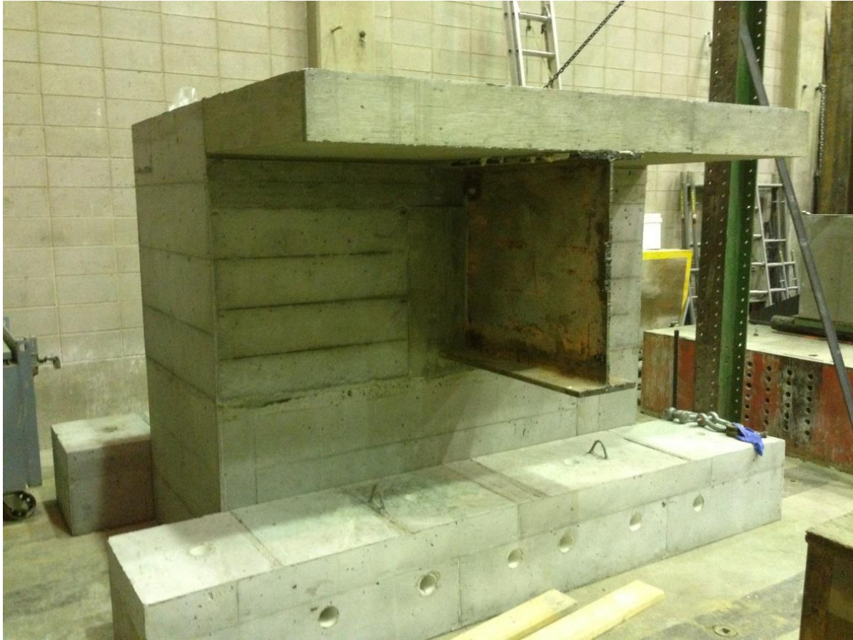
Figure 22. Cast-in-place integral abutment specimen
