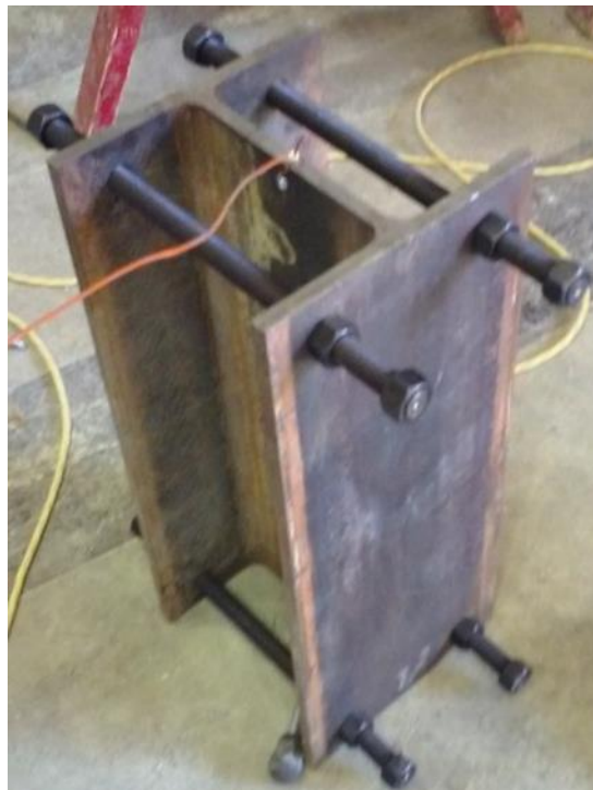
Figure 42. HP section with threaded rods
