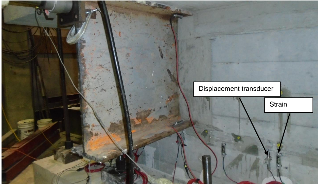
Figure 62. Front face of the abutment during horizontal loading
