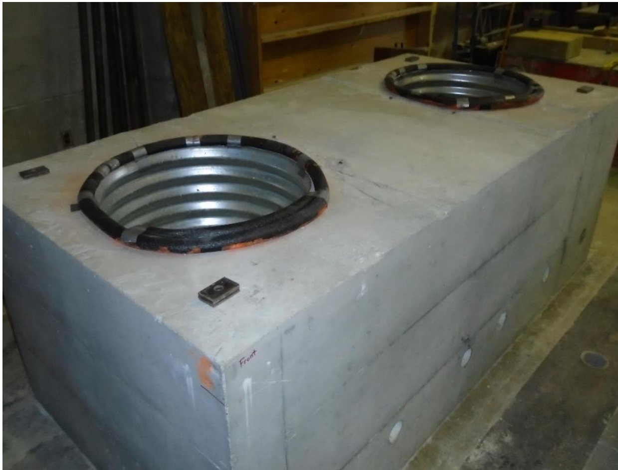
Figure 48. Pile cap with backer rod seal
