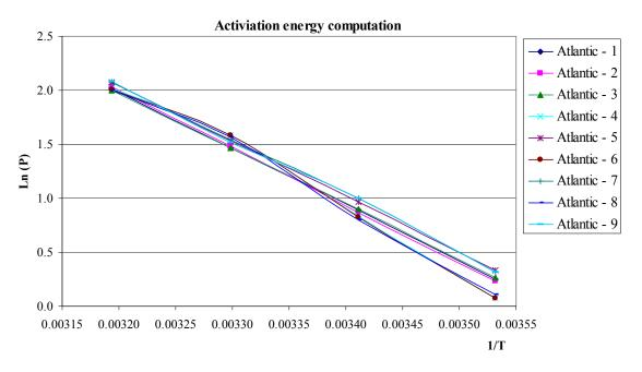
Figure 69. Activation energy calculation for Atlantic site (nine mixes, at four temperatures: 10 °C, 20 °C, 30 °C, and 40 °C; P unit: mW/g; T unit: K).
