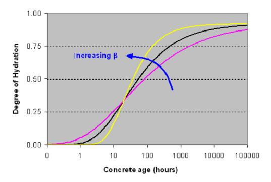
Figure 74. Influence of hydration curve parameter **t** on degree of hydration
