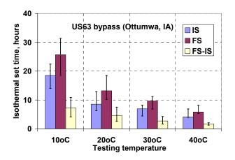
Figure 57. Estimated set time from isothermal robust test on US 63 bypass (Ottumwa, IA) mixes
