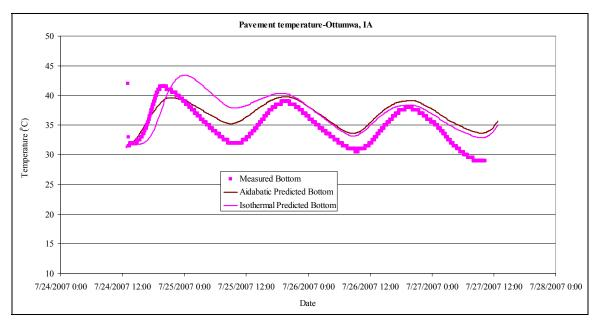
Figure 112. Predicted pavement temperatures versus measurements (pavement bottom, Ottumwa, IA)
