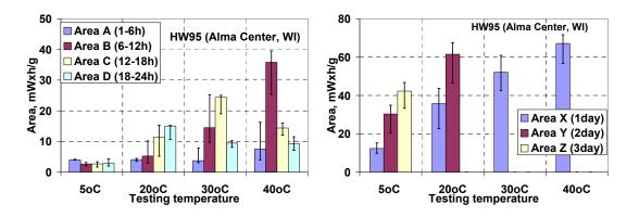
Figure 47. Heat generation from isothermal robust test mixes at different times HW95 (Alma Center, WI) mixes
