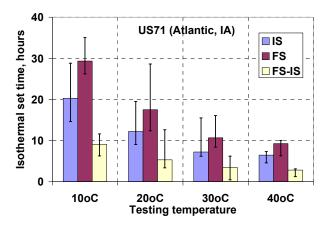
Figure 36. Estimated set time from isothermal robust test on US 71 (Atlantic, IA) mixes
