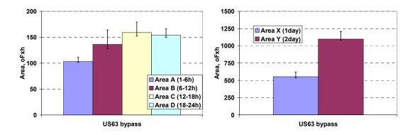
Figure 53. Areas under AdiaCal test curves of US 63 bypass (Ottumwa, IA) projects during different test period
