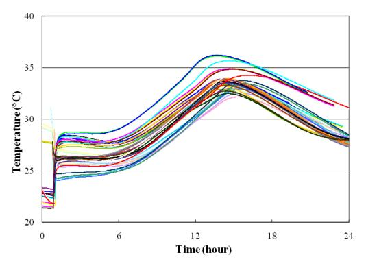
Figure A.1. Concrete temperature for all samples for Atlantic project
