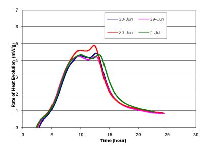
Figure 9. Isothermal calorimetry results for US 71 (Atlantic, IA) field concrete samples
