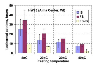
Figure 46. Estimated set time from isothermal robust test on HW 95 (Alma Center, WI) mixes
