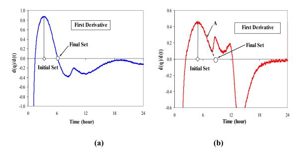
Figure E.1. Determination of set times from heat evolution curve
