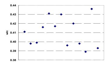
Figure 4. Water to cement ratio for the mixes of US 71 (Atlantic project)
