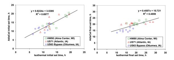
Figure 64. Comparison of isothermal and AdiaCal set time results
