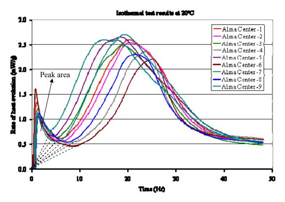
Figure 75. Pre-process the data of rate of heat evolution from isothermal tests
