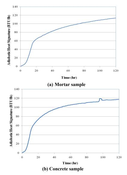
Figure 10. Heat evolution with time for US 71 (Atlantic, IA) field test
