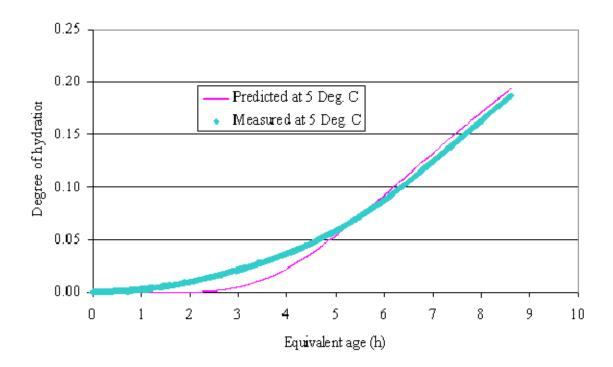
Figure 77. Predicted degree of hydration vs. measurements at 5 °C (Sample 5, Alma Center)
