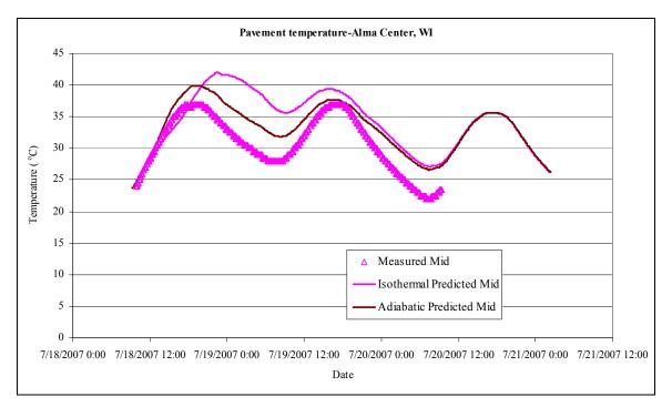
Figure 99. Predicted pavement temperatures versus measurements (pavement mid, Alma Center, WI)
