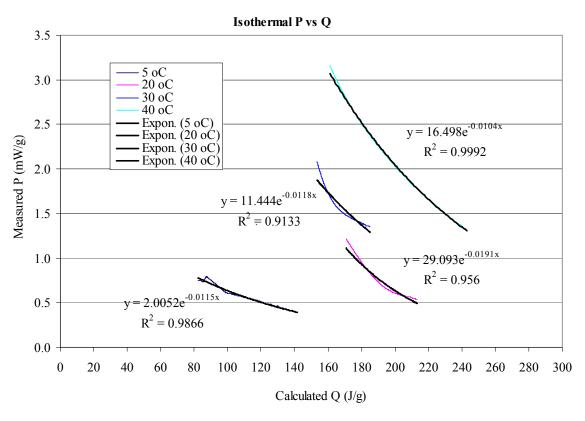
Figure 86. Exponential equations to approximate P vs. Q
