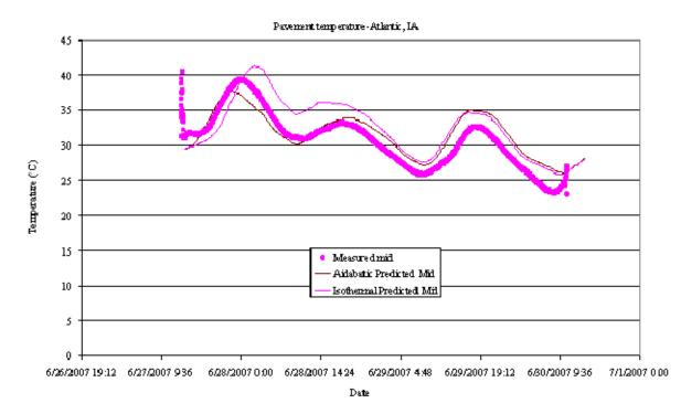
Figure 105. Predicted pavement temperatures versus measurements (pavement mid, Atlantic, IA)
