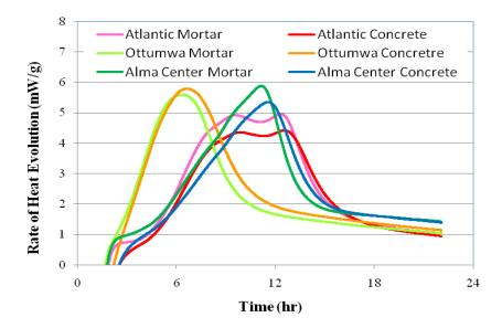
Figure 28. Summary of isothermal field calorimetry results
