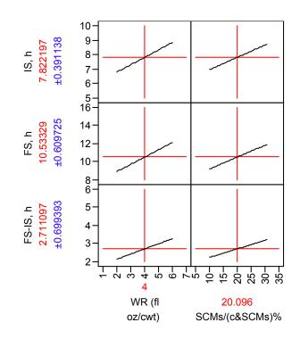
Figure 61. Effect of mix design on ASTM setting time US63 bypass (Ottumwa, IA) mixes
