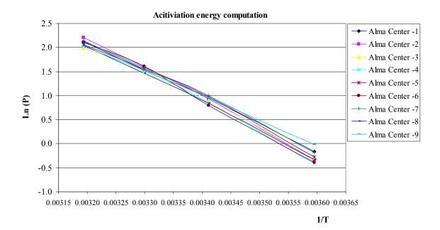
Figure 68. Activation energy calculation for AlmaCenter site (nine mixes, at four temperatures: 5 °C, 20 °C, 30 °C, and 40 °C; P unit: mW/g; T unit: K).
