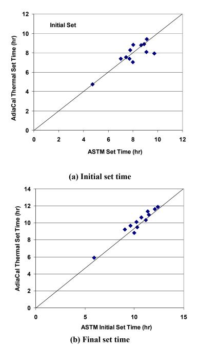
Figure 15. ASTM set time vs. AdiaCal thermal set for HW 95 (Alma Center, WI) project, 18% fraction for initial thermal set and 41% for final thermal set
