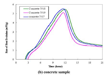
Figure 17. Isothermal calorimetry results from HW 95 (Alma Center, WI) field study
