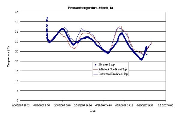
Figure 104. Predicted pavement temperatures versus measurements (pavement top, Atlantic, IA)
