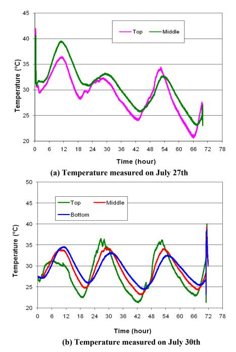
Figure 12. Pavement temperature from US 71 (Atlantic, IA) field tests
