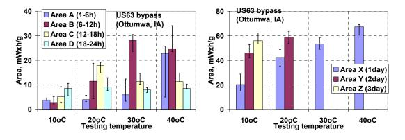
Figure 58. Heat generation from isothermal robust test mixes at different times US 63 bypass (Ottumwa, IA) mixes
