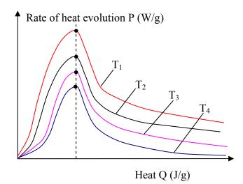
Figure 66. Locate maximum hydration rate
