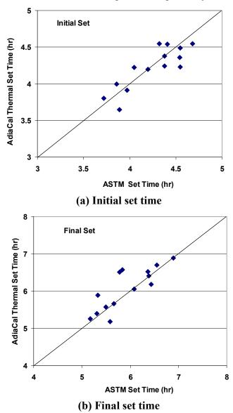
Figure 22. ASTM set time vs. AdiaCal thermal set for US 63 bypass (Ottumwa, IA) project—13% fraction for initial thermal set and 49% for final thermal set
