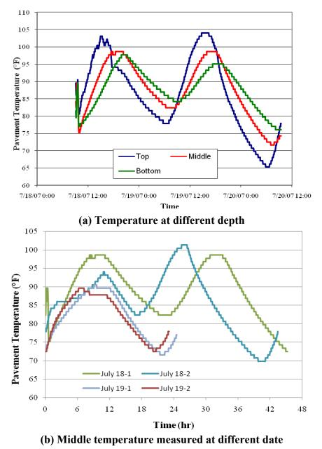
Figure 20. Pavement temperature for HW 95 (Alma Center, WI) project
