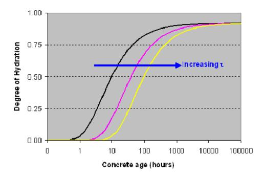
Figure 73. Influence of hydration curve parameter β on degree of hydration
