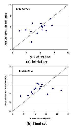
Figure 7. ASTM set time vs. AdiaCal thermal set time from US 71 (Atlantic, IA) field study (Initial thermal set—17% and 14% fraction for two AdiaCal, respectively; Final thermal set—50% fraction for both AdiaCal)
