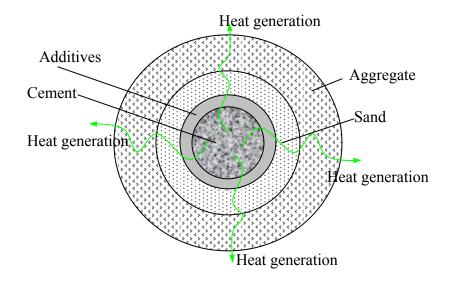
Figure 91. Heat generation of cementitious material
