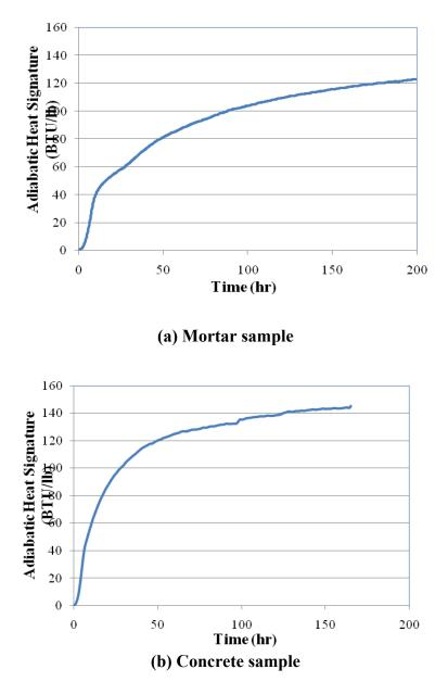
Figure 24. Heat evolution with time for US 63 bypass (Alma Center, WI) project
