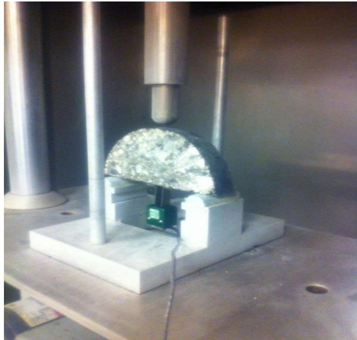
Figure 5-17: A Typical Specimen under SCB Test Machine
