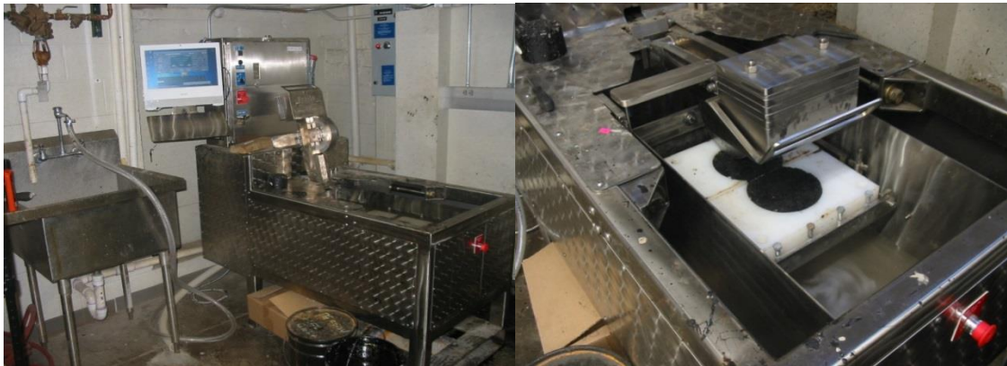
Figure 5-1: Hamburg Wheel Tracking Device and Specimens ready for testing
