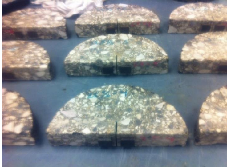
Figure 5-16: Specimens for SCB Test
