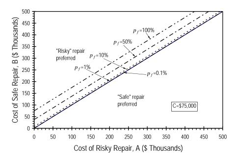
Figure 4.4. Family of break-even lines for different assumed values of  $p_f$
