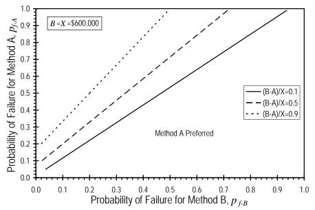
Figure 4.13. Break-even lines determined using the constant-method STH model for a fiveyear time horizon with B=X=\$600,000
