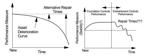
Figure 2.3. Asset deterioration curves: (a) Traditional pavement deterioration and (b) Deterioration of an embankment over soft foundation soils.
