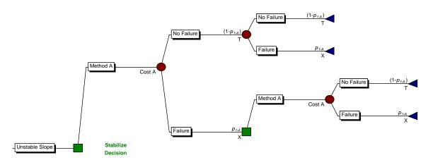
Figure 4.12. Method A branch of constant-method Specific Time Horizon model for twoyear time horizon
