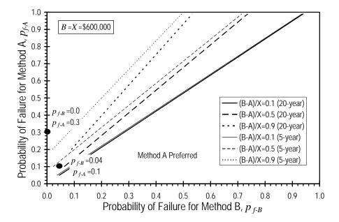
Figure 4.17. Application of constant-method STH model for two example problems based on input from ODOT database
