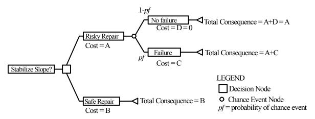
Figure 4.1. Example of a simple decision tree modeling the slope repair problem
