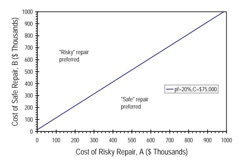
Figure 4.2. Break-even relation for simple decision tree of Figure 4.1 for C=\$75,0000, D=\$0, and  $p_f=20\%$
