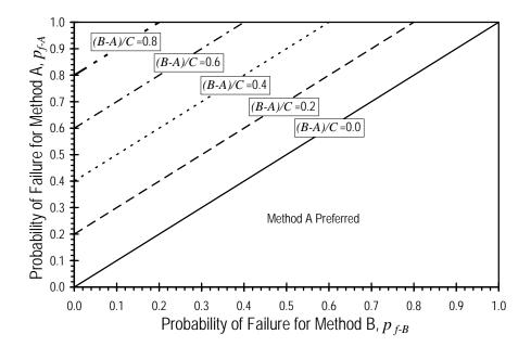
Figure 4.6. Break-even lines for Basic IIT Model in terms of  $p_{f-A}$  and  $p_{f-B}$
