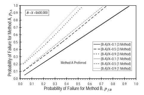
Figure 4.15. Comparison of break-even lines determined for a time horizon of 5 years using the three-method and constant-method STH models
