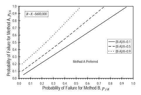
Figure 4.11. Break-even lines determined using the three-method STH model for a fiveyear time horizon with B=X=\$600,000
