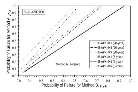
Figure 4.16. Comparison of break-even lines determined for time horizons of 5 and 20 years using the constant-method STH model
