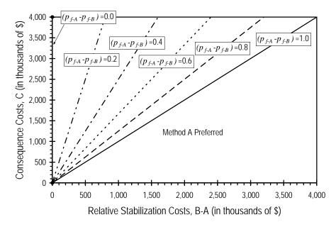
Figure 4.7. Break-even lines for Basic IIT Model in terms of (B-A) and C
