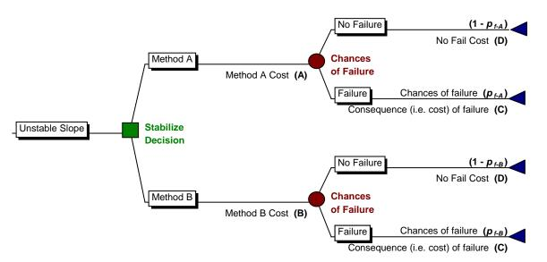
Figure 4.5. Basic Instant in Time model representing the slope repair problem
