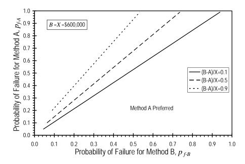
Figure 4.14. Break-even lines determined using the constant-method STH model for a twenty-year time horizon with *B*=*X*=\$600,000
