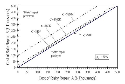
Figure 4.3. Family of break-even lines for different assumed values of C
