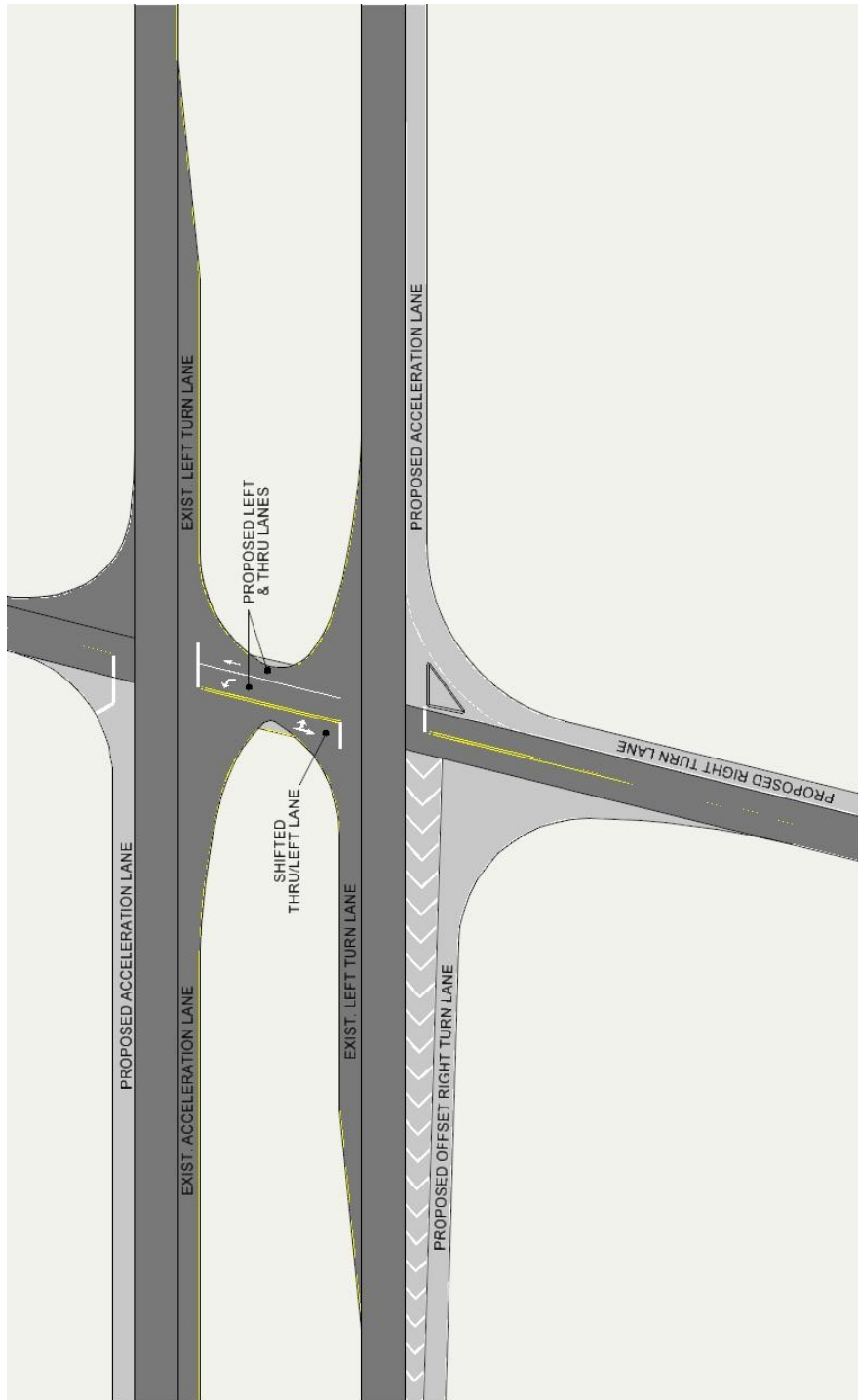
Figure F.1.1. Median turn-lane option with proposed offset right-turn and acceleration lanes
