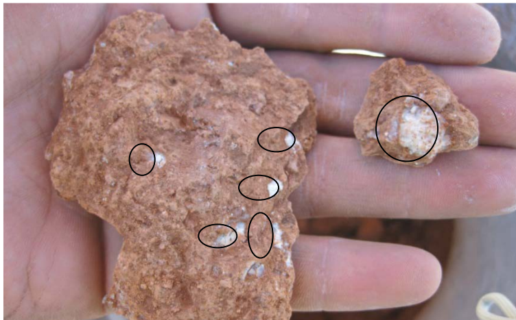
Figure 9. White product presented in stabilized subgrade at test site of US 183
