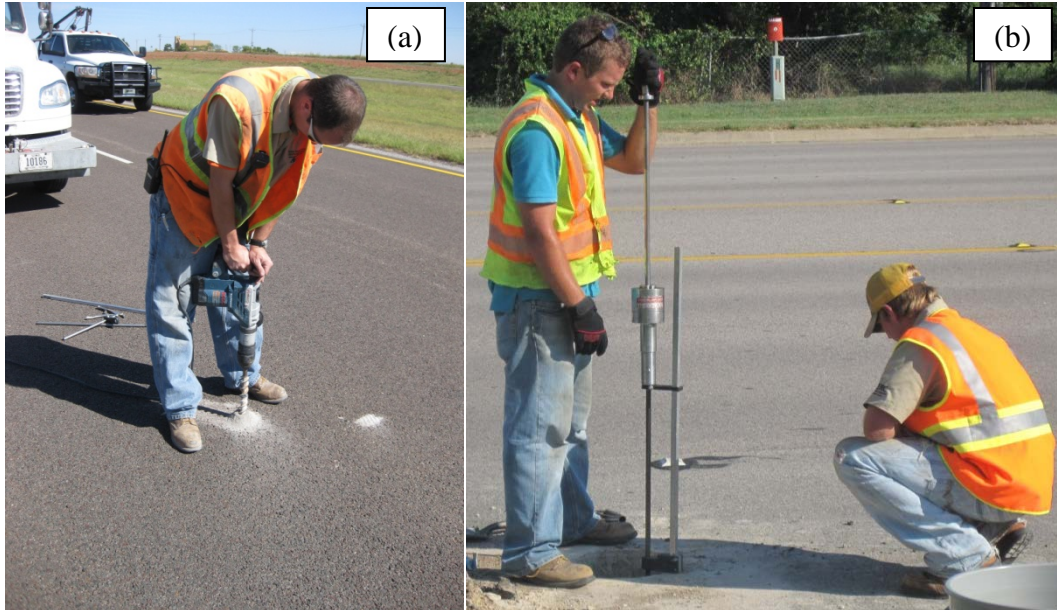
Figure 1. (a) Drilling 1.5 inch diameter hole prior to DCP test, (b) dynamic cone penetrometer test
