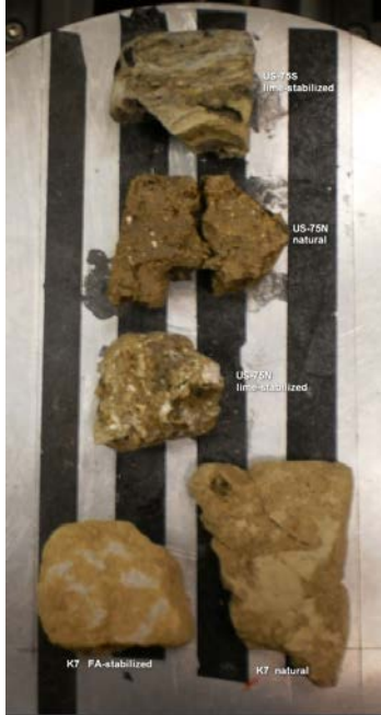
Figure 8. Prepared SEM samples from test sites in Kansas
