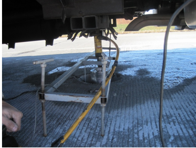
Figure 4. Plate load test in core hole.
