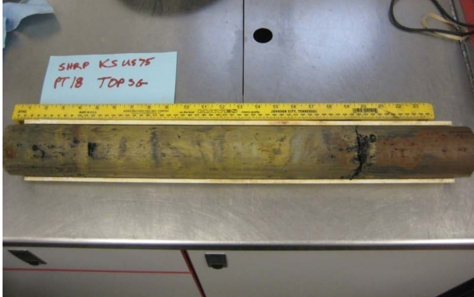
Figure 7. Example of Shelby tube sample after extraction
