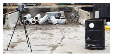
Laser scanning a concrete cylinder
