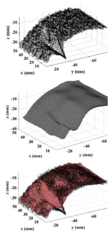
Process of fitting the point cloud data to the representation created by the wavelet neural network with point cloud data (top), compact representation (center), and overlap of point cloud and representation (bottom)
