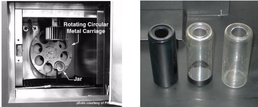
Figure 3.7. The RTFO Chamber and the Sample Cylinders
