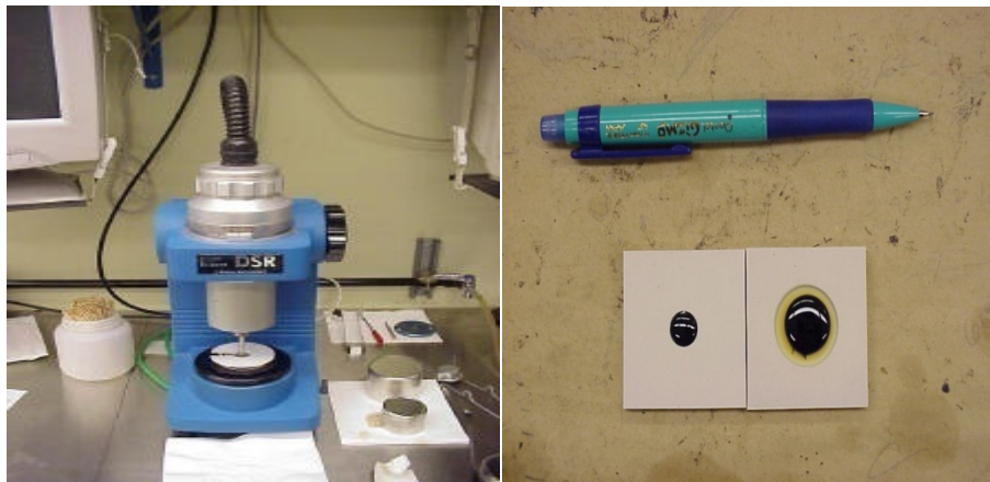
Figure 3.9. Dynamic Shear Rheometer Machine and the Sample
