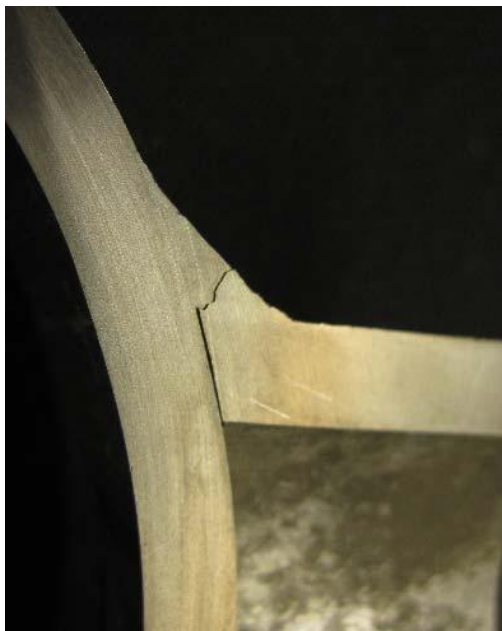
(a). Crack at throat
