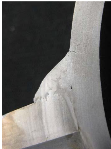
(b). Crack at toe
