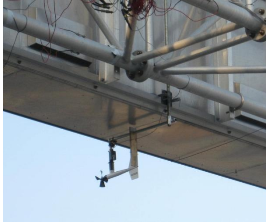
Fig. 30. View of an anemometer mounted underneath the DMS cabinet
