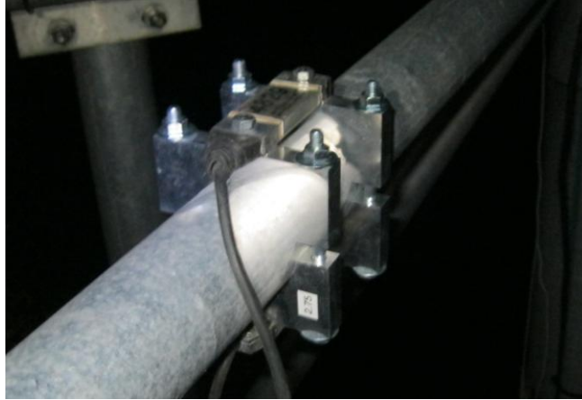
Fig. 28 View of a strain gage attached on a small member of the truss
