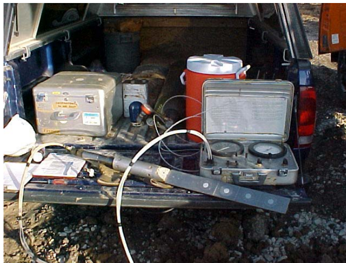
Figure 26. K_o Stepped Blade Test Equipment
