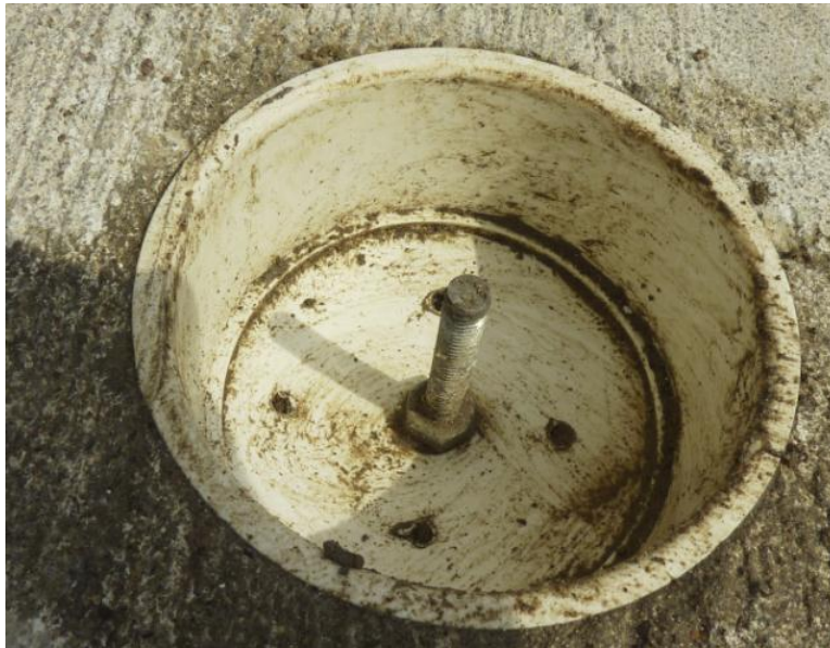
Figure 66. View of embedded coupon holder with mounting bolt
