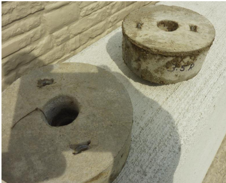
Figure 64. Closeup of coupon samples removed from paved shoulder locations
