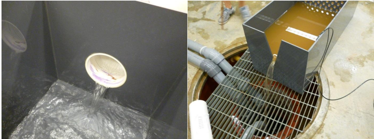
Figure 42. Pressure transducer placement in weir box
