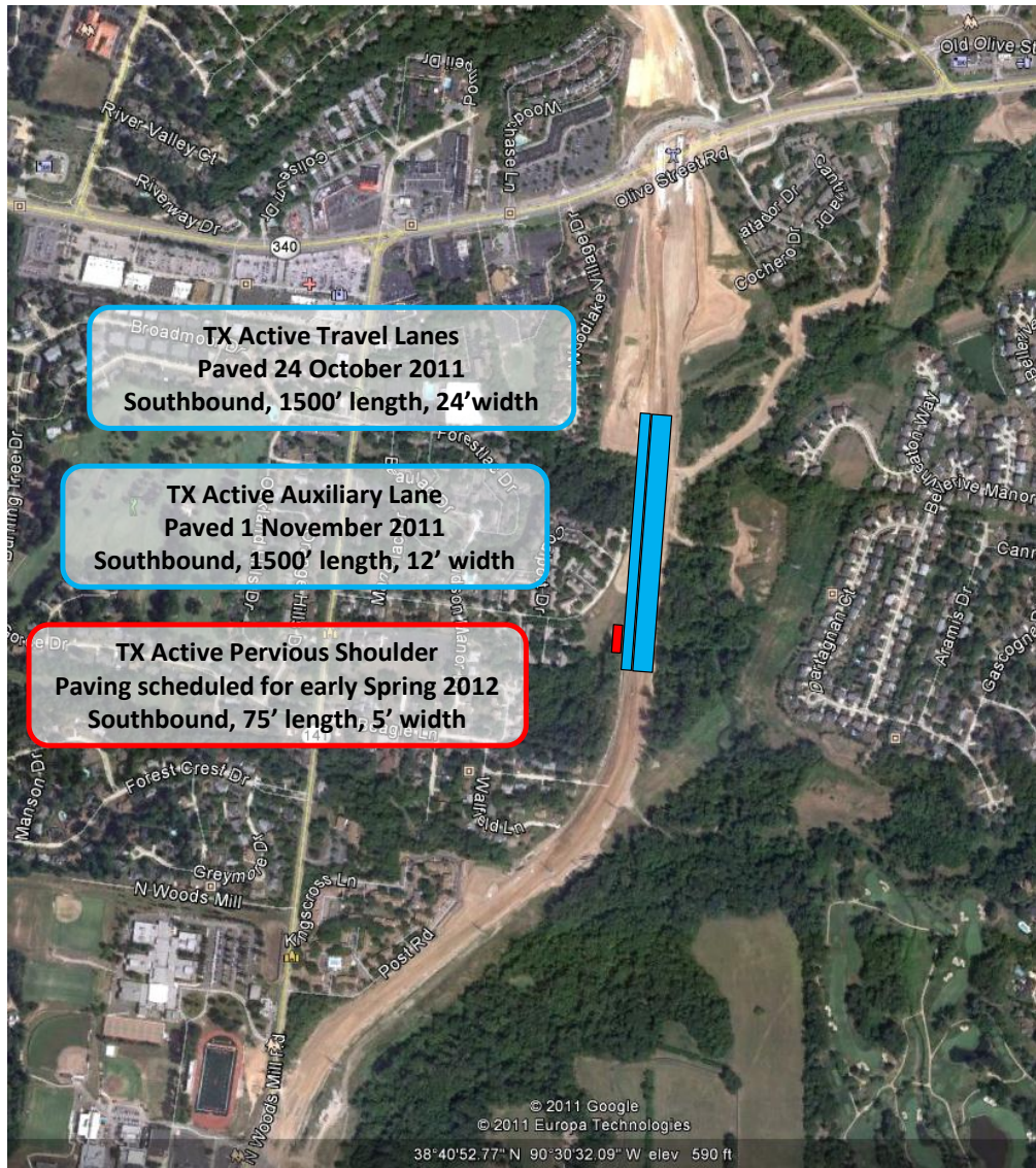
Figure 30. Paving overview with top TX Active layer in foreground
