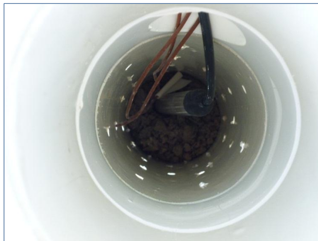
Figure 52. Perforated stand pipe within aggregate base showing pressure sensor and thermocouple wires
