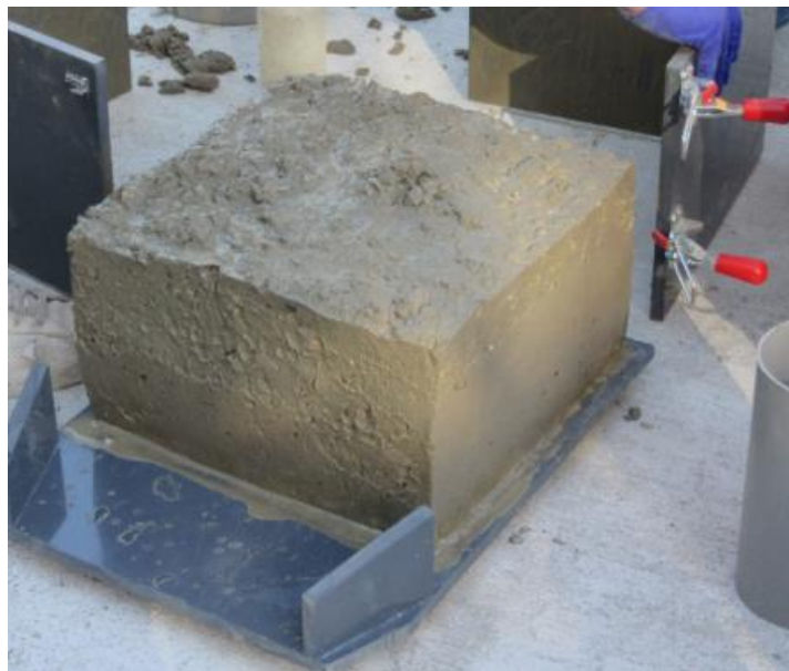
Figure 6. Mix 2 Set 1 box test showing an edge slump
