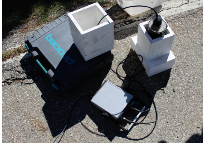
Figure 9. UPV test setup with sample in a wooden frame for stability
