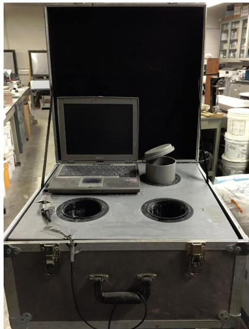
Figure 8. Calorimetry test device for measuring the heat of hydration of concrete
