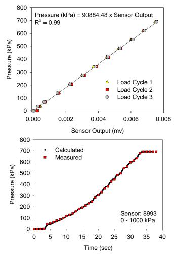
Figure 12. EPC calibration test results (sensor 8993)
