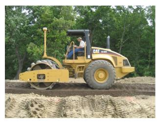
Figure 19. Caterpillar CS563 padfoot vibratory roller
