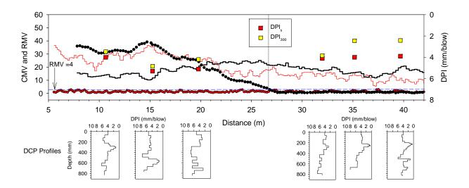
Figure 29. Comparison of CMV / RMV to DCP measurement values
