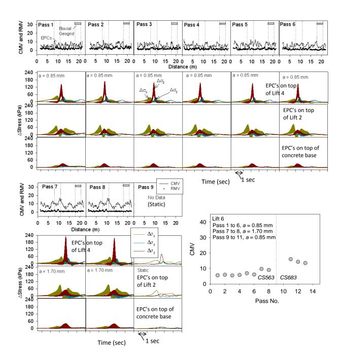
Figure 54. CMV and in-ground stress measurements for CS 563 roller passes – lift 6
