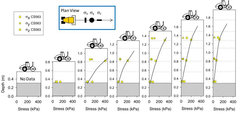
Figure 81. Stress distribution under the roller at a = 1.70 mm – TB 2
