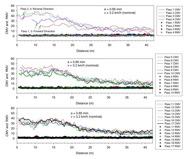
Figure 22. CMV and RMV data plots for pass 1 to 17 using CS 563 roller at *a* = 0.85 mm
