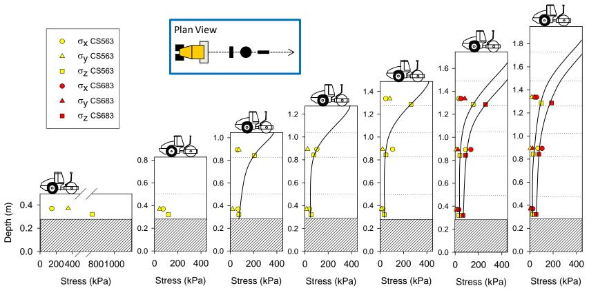
Figure 58. Stress distribution under the roller at a = 0.85 mm – TB 1
