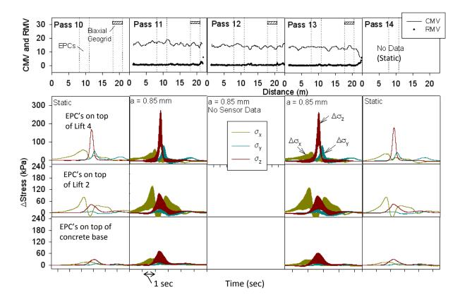
Figure 55. CMV and in-ground stress measurements for CS 683 roller passes – lift 6
