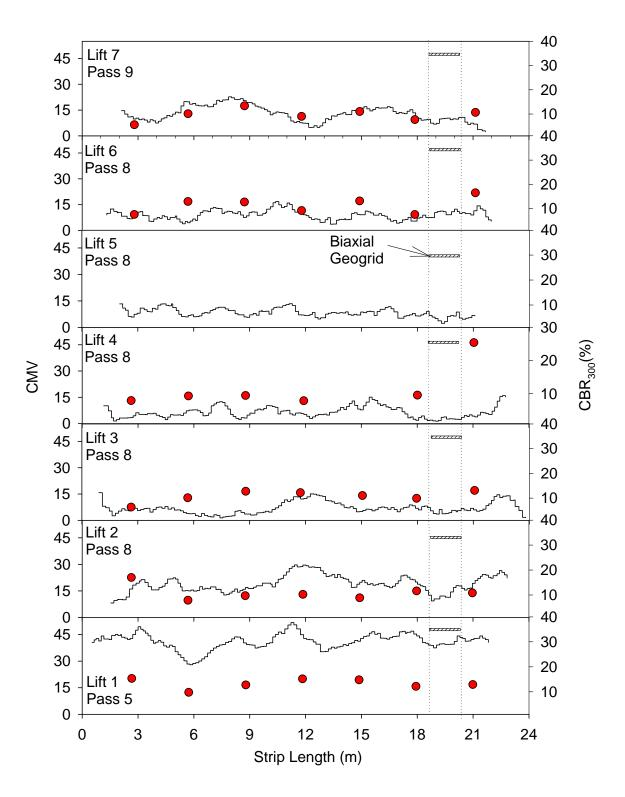
Figure 62. CMV and CBR measurement values after final pass on each lift – TB 1
