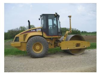
Figure 17. Caterpillar CS563 smooth drum vibratory roller
