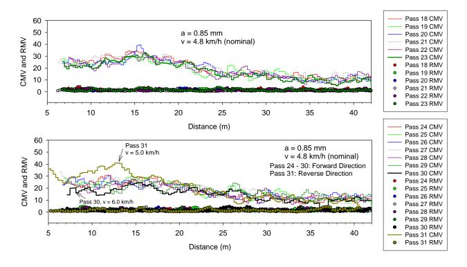
Figure 23. CMV and RMV data plots for pass 18 to 31 using CS 563 roller at *a* = 0.85 mm
