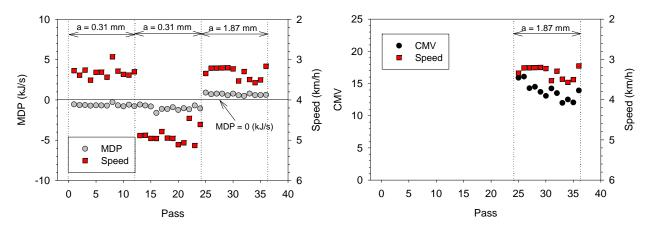
Figure 31. Summary of average MDP, CMV, and speed of operation for several passes on repeatability test strip 2
