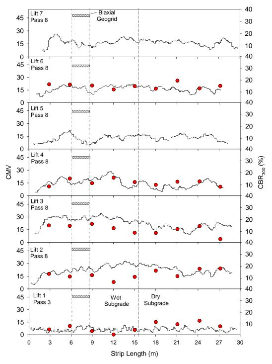
Figure 78. CMV and CBR measurement values after final pass on each lift – TB 2
