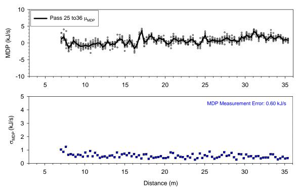
Figure 43. Repeatability analysis for CP 563 MDP measurement values at a = 1.87 mm and v = 3.2 km/h (nominal)
