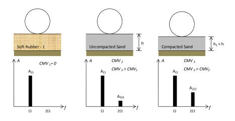
Figure 2. Illustration of relationship between subsurface conditions and CMV
