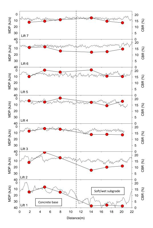
Figure 96. MDP and CBR comparison plot after final pass on each lift – TB 3
