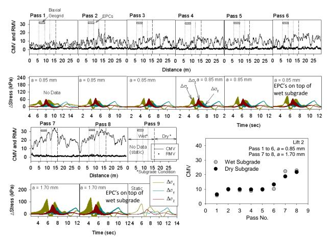
Figure 71. CMV and in-ground stress measurements for CS 563 roller passes – lift 2
