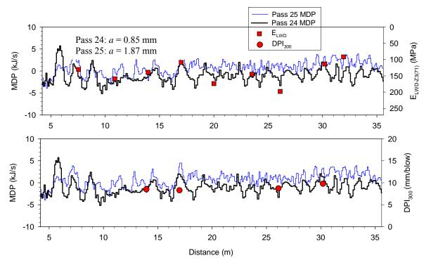
Figure 34. Comparison between MDP and in-situ compaction test measurement values
