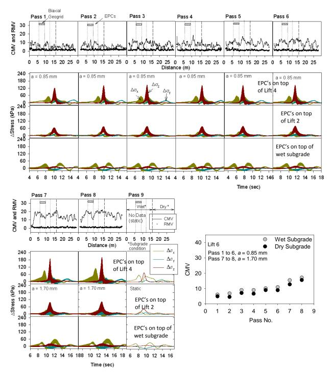
Figure 75. CMV and in-ground stress measurements for CS 563 roller passes – lift 6
