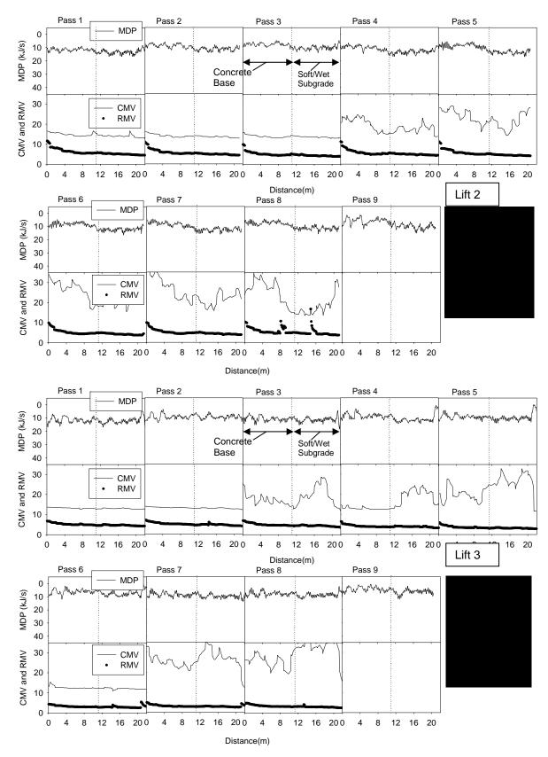
Figure 88. Raw data plots of MDP, CMV, and RMV measurements on lifts 2 and 3
