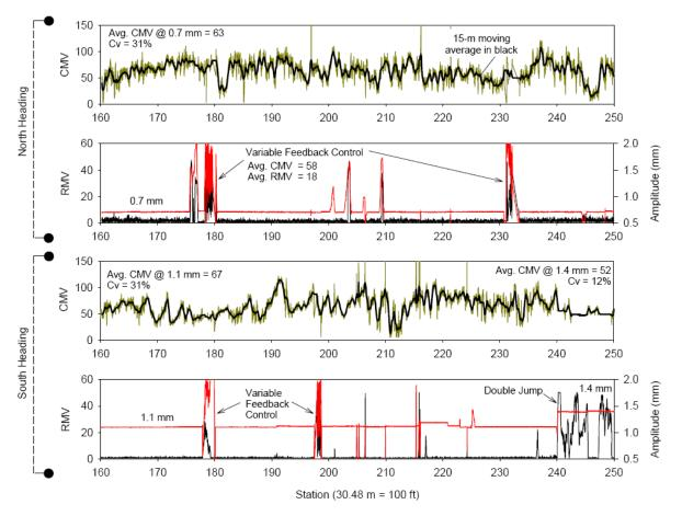
Figure 7. CMV, RMV, amplitude data for 2.7 km test section (White et al. 2008)
