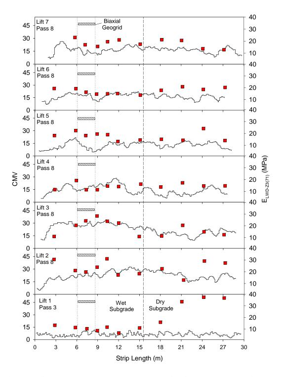
Figure 77. CMV and  $E_{LWD}$  measurement values after final pass on each lift – TB 2  $\,$
