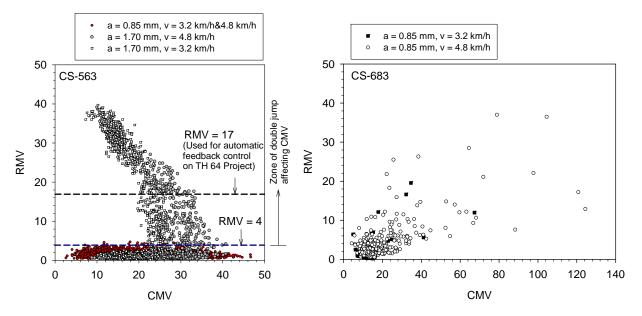
Figure 27. CMV and RMV comparison plots to define double jump and partial uplift zones for CS-563 and CS-683 rollers
