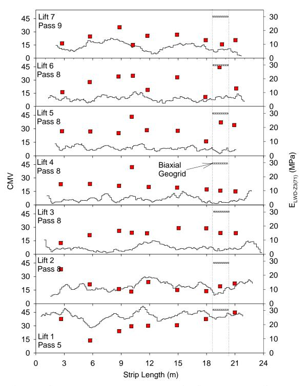
Figure 61. CMV and  $E_{LWD}$  measurement values after final pass on each lift – TB 1
