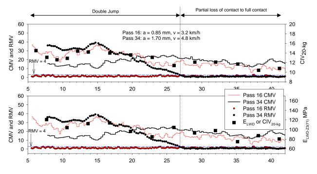
Figure 28. Comparison of CMV / RMV to  $E_{LWD}$  and CIV measurement values
