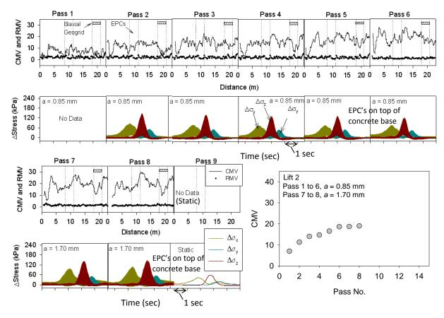
Figure 50. CMV and in-ground stress measurements for CS 563 roller passes – lift 2
