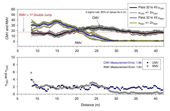
Figure 38. Repeatability analysis for CS 563 CMV/RMV measurement values at a = 1.70 mm and v = 3.2 km/h (nominal)
