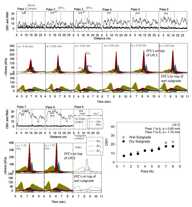
Figure 72. CMV and in-ground stress measurements for CS 563 roller passes – lift 3
