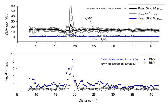
Figure 40. Repeatability analysis for CS 683 CMV/RMV measurement values at a = 0.85 mm and v = 3.2 km/h (nominal)
