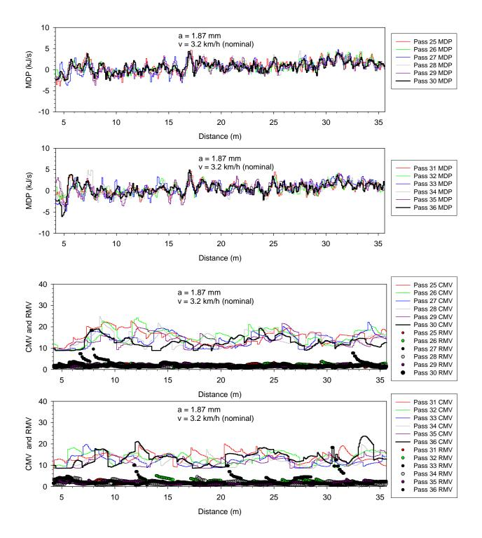
Figure 33. MDP and CMV raw data plots for pass 25 to 36 using CP 563 (padfoot) roller at a = 1.87 mm
