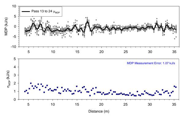
Figure 42. Repeatability analysis for CP 563 MDP measurement values at a = 0.31 mm and v = 4.8 km/h (nominal)
