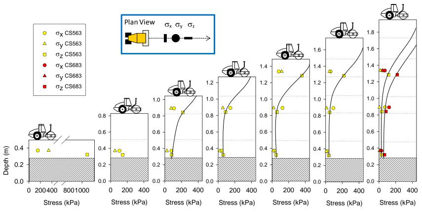
Figure 59. Stress distribution under the roller at a = 1.70 mm – TB 1
