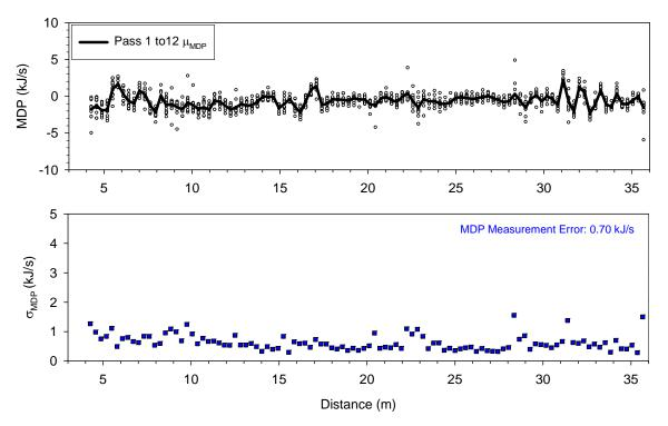
Figure 41. Repeatability analysis for CP 563 MDP measurement values at a = 0.31 mm and v = 3.2 km/h (nominal)
