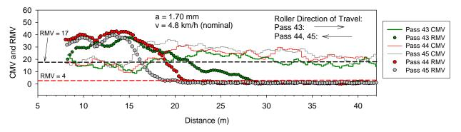
Figure 25. CMV and RMV data plots for pass 43 to 45 using CS 563 roller at *a* = 1.70 mm
