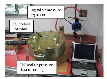
Figure 11. Complete setup of the EPC calibration chamber
