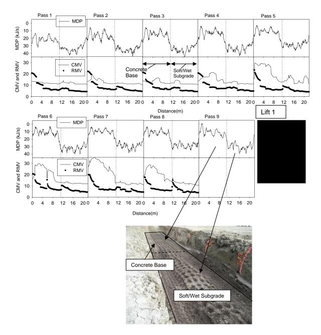
Figure 87. Raw data plots of MDP, CMV, and RMV measurements on lift 1 (picture showing the rutting observed on lift 1 after pass 9)
