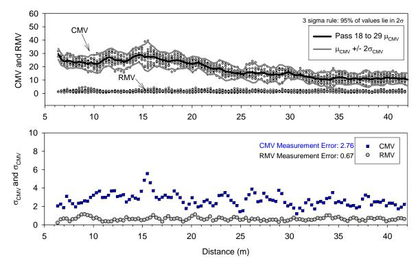
Figure 37. Repeatability analysis for CS 563 CMV/RMV measurement values at a = 0.85mm and v = 4.8 km/h (nominal)
