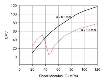
Figure 6. Influence of amplitude on CMV in relationship to soil stiffness based on numerical simulations (reproduced from Sandström 1994)
