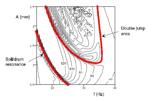
Figure 4. Variation of CMV with frequency and amplitude of the roller for constant soil conditions (Shear Modulus, G = 80 MPa, and plastic deformation, p = 0.5 mm) (modified from Sandström (1994))
