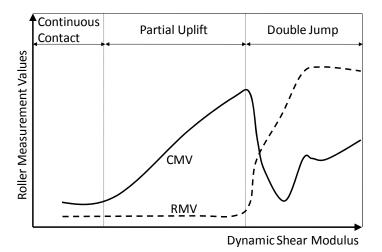
Figure 5. CMV and RMV change with drum behavior and soil stiffness based on numerical simulations (reproduced from Adam 1996)
