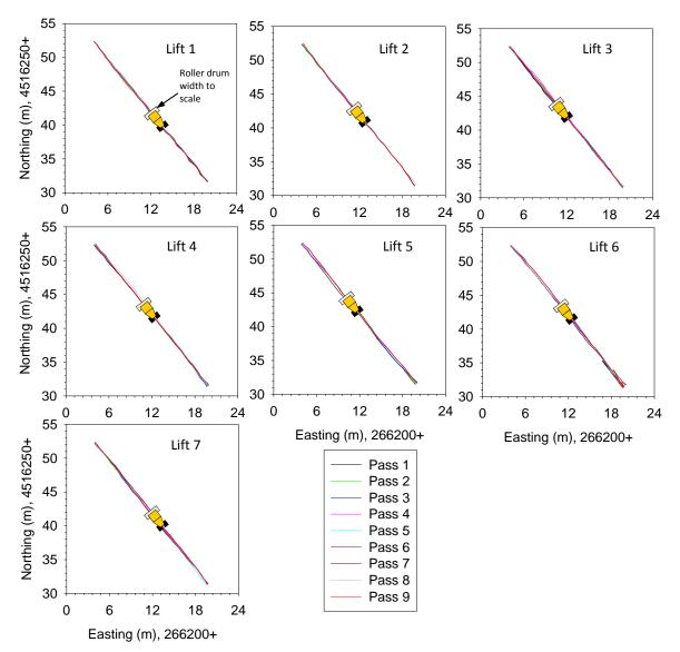
Figure 94. GPS position of roller drum during compaction passes on each lift – TB 3 (color)
