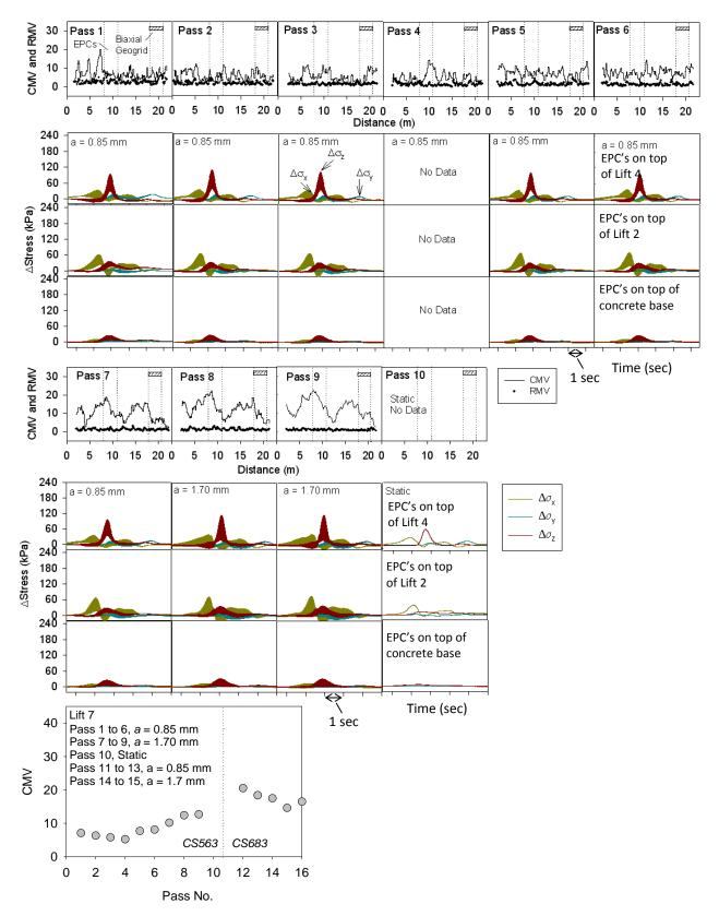
Figure 56. CMV and in-ground stress measurements for CS 563 roller passes – lift 7
