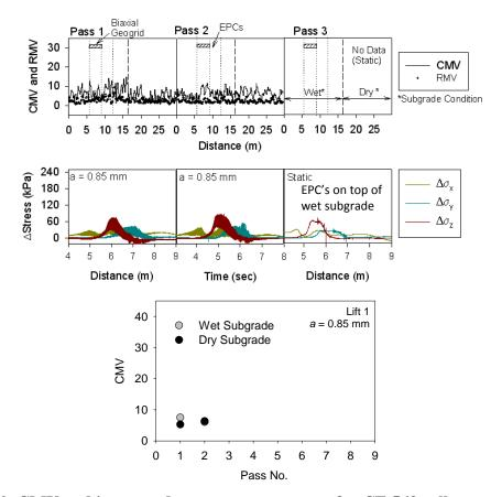
Figure 70. CMV and in-ground stress measurements for CE 563 roller passes – lift 1
