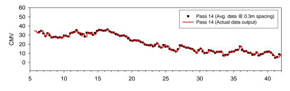
Figure 35. Comparison of actual CMV data output and 0.305 m (1 ft.) averaged data
