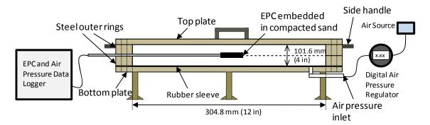
Figure 9. Schematic cross-section of the EPC calibration chamber
