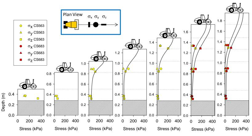
Figure 60. Stress distribution under the roller in static mode – TB 1
