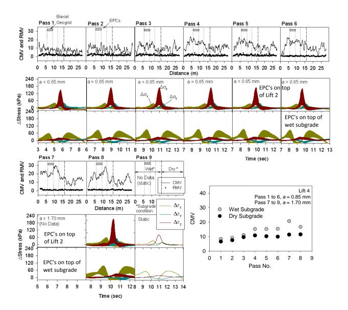
Figure 73. CMV and in-ground stress measurements for CS 563 roller passes – lift 4
