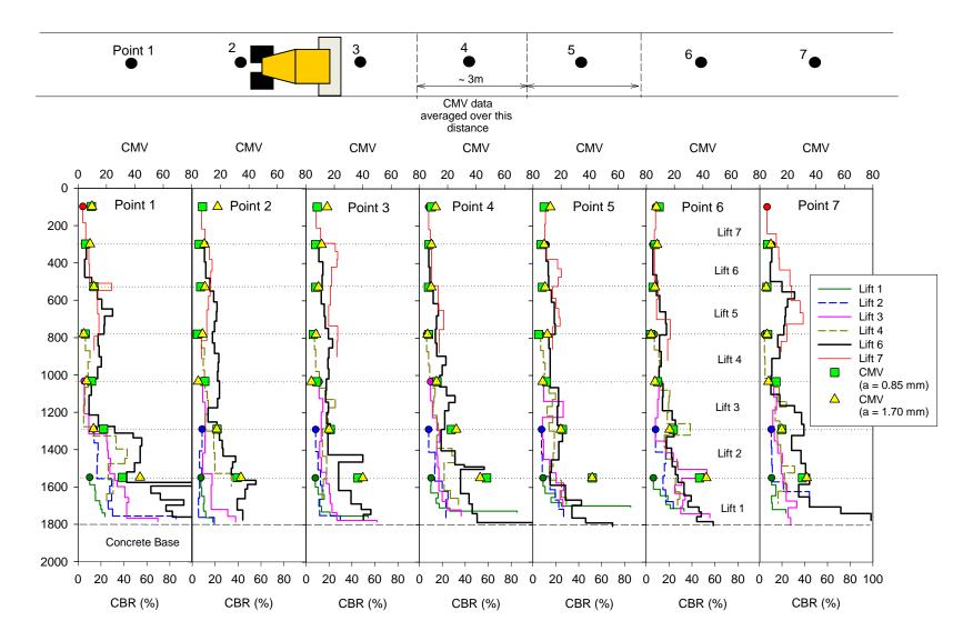
Figure 64. DCP-CBR profiles on each lift at seven points along the test bed with comparison to CMV measurements on each lift
