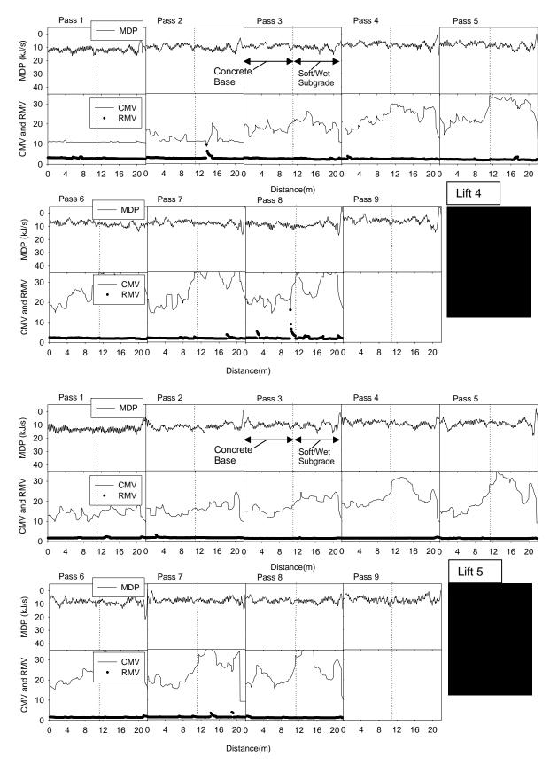
Figure 89. Raw data plots of MDP, CMV, and RMV measurements on lifts 4 and 5
