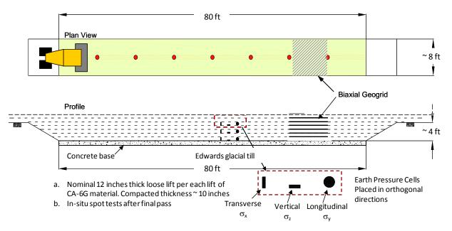
Figure 44. TB 1 plan view and profile with location of in-ground EPCs
