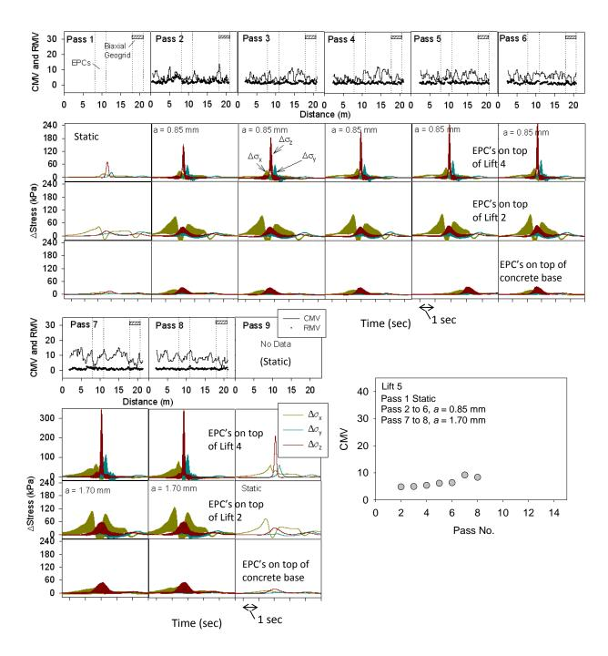
Figure 53. CMV and in-ground stress measurements for CS 563 roller passes – lift 5
