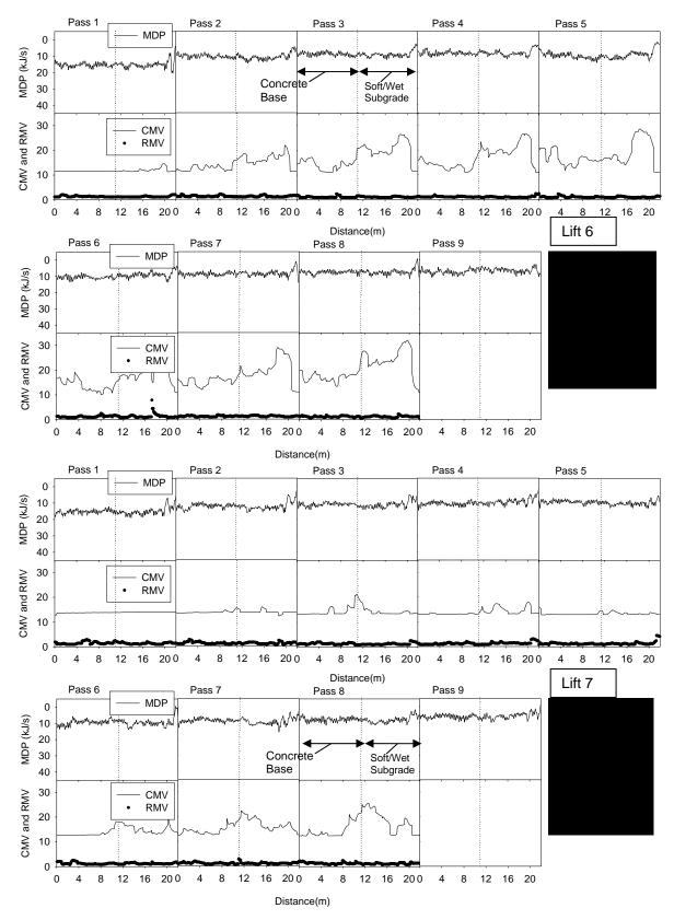
Figure 90. Raw data plots of MDP, CMV, and RMV measurements on lifts 6 and 7
