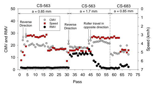
Figure 21. Summary of average CMV and speed of operation for test strip 1
