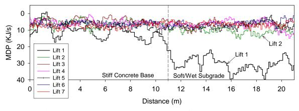
Figure 92. Pass 9 MDP measurements on lifts 1 to 7 – TB 3 (color)
