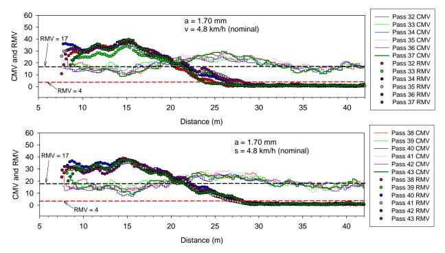
Figure 24. CMV and RMV data plots for pass 32 to 43 using CS 563 roller at *a* = 1.70 mm
