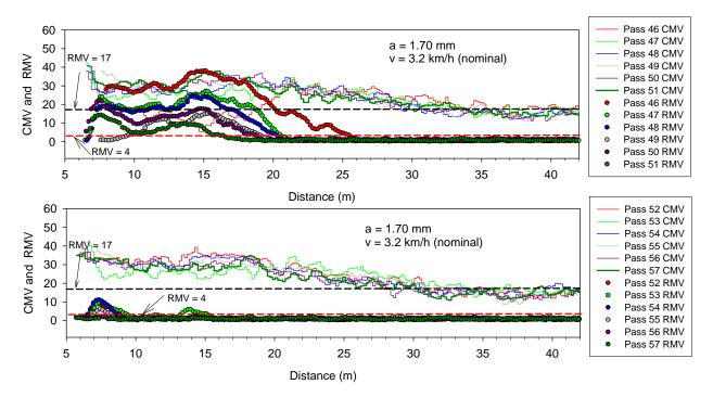
Figure 26. CMV and RMV data plots for pass 46 to 57 using CS 563 roller at *a* = 1.70 mm
