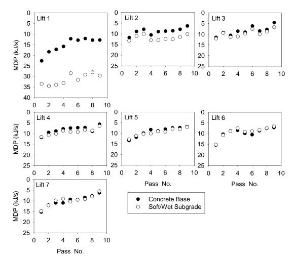
Figure 93. MDP compaction growth curves – TB 3
