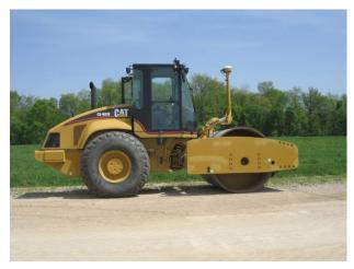
Figure 18. Caterpillar CS683 smooth drum vibratory roller
