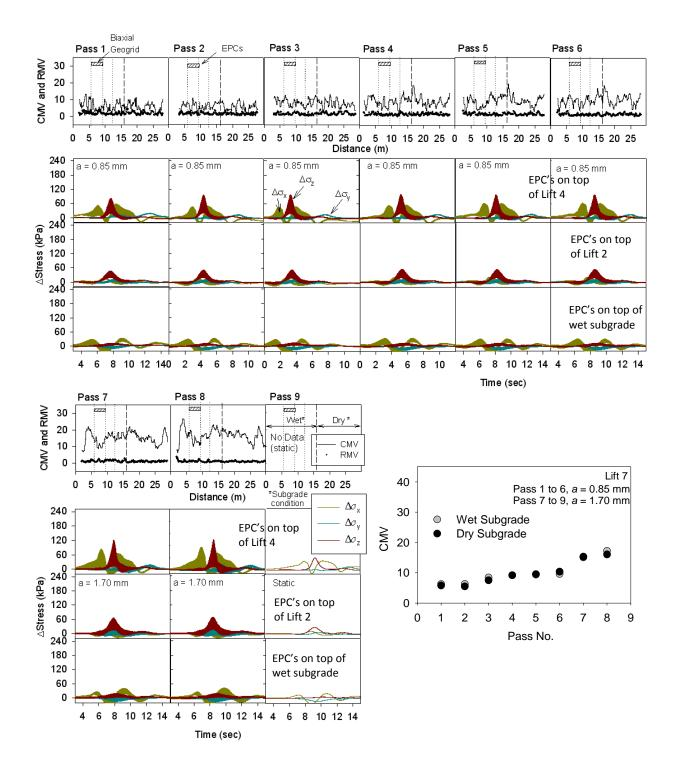
Figure 76. CMV and in-ground stress measurements for CS 563 roller passes - lift 7
