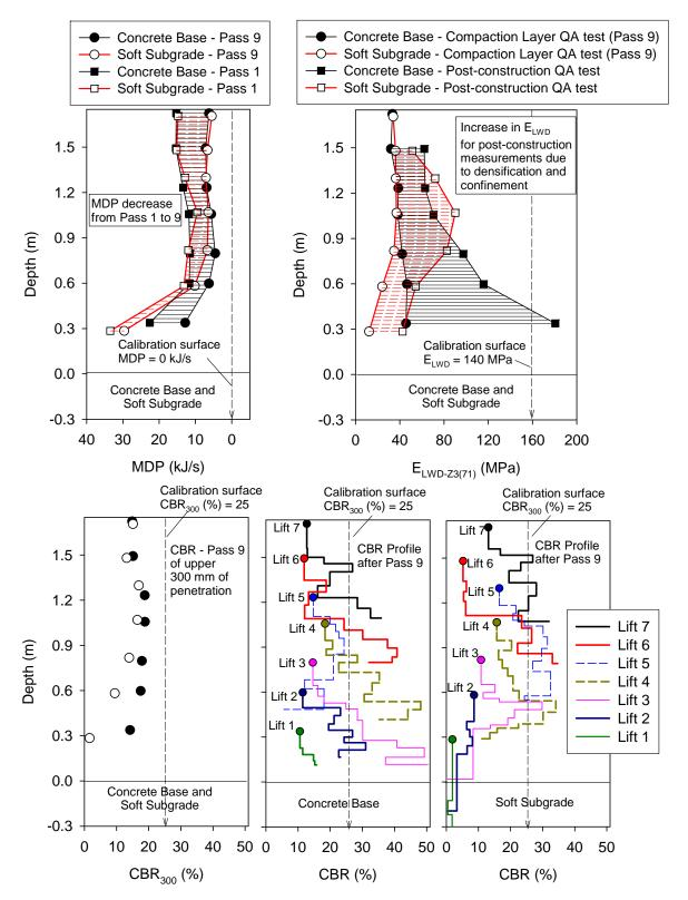
Figure 98. Average MDP,  $E_{LWD}$ , and CBR measurement values on all compaction lifts – TB3
