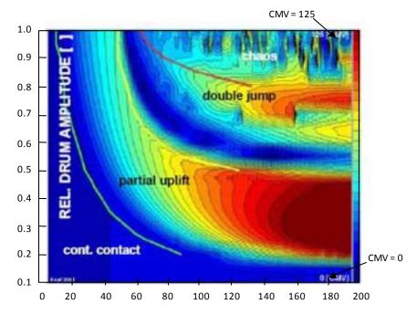
Figure 3. Variation in CMV with change in elastic modulus of the soil and relative vertical amplitude at excitation frequency f = 28 Hz (modified from Adam and Kopf 2004)
