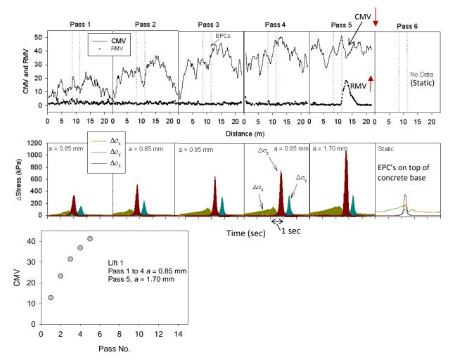
Figure 49. CMV and in-ground stress measurements for CS 563 roller passes – lift 1
