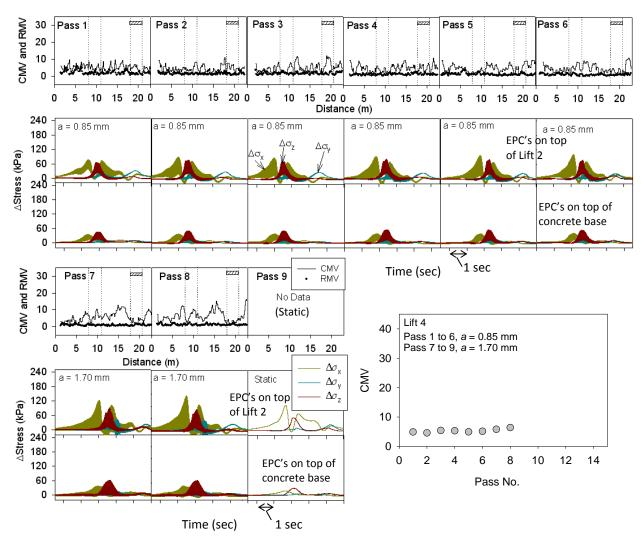
Figure 52. CMV and in-ground stress measurements for CS 563 roller passes – lift 4
