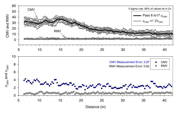
Figure 36. Repeatability analysis for CS 563 CMV/RMV measurement values at a = 0.85mm and v = 3.2 km/h (nominal)
