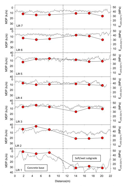
Figure 95. MDP and  $E_{LWD}$  comparison plot after final pass on each lift – TB 3
