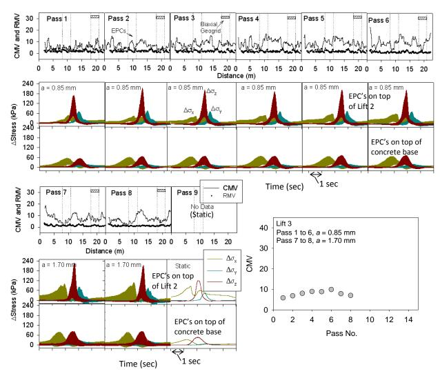
Figure 51. CMV and in-ground stress measurements for CS 563 roller passes – lift 3
