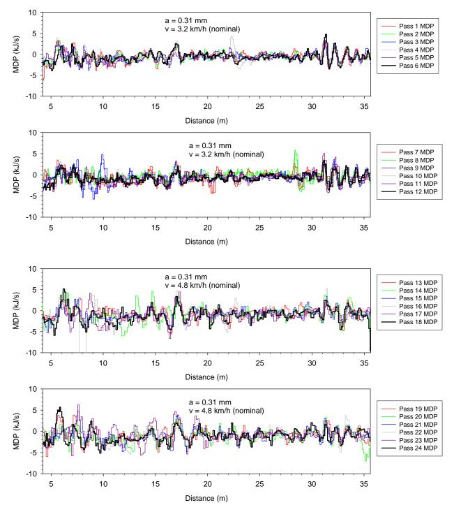
Figure 32. MDP raw data plots for pass 13 to 24 using CP 563 (padfoot) roller at *a* = 0.31 mm
