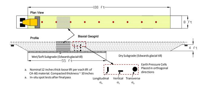
Figure 65. TB 2 plan view and profile with in-ground EPC's
