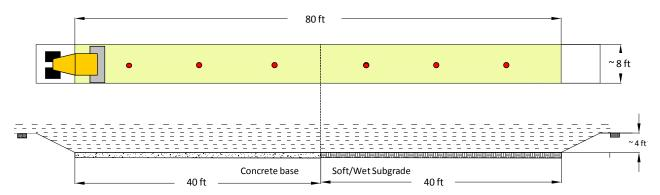
Figure 83. TB 3 plan view and profile with location of in-ground EPCs
