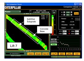
Figure 91. Caterpillar viewer program screen shots of MDP final static pass on each lift – TB 3 (color)
