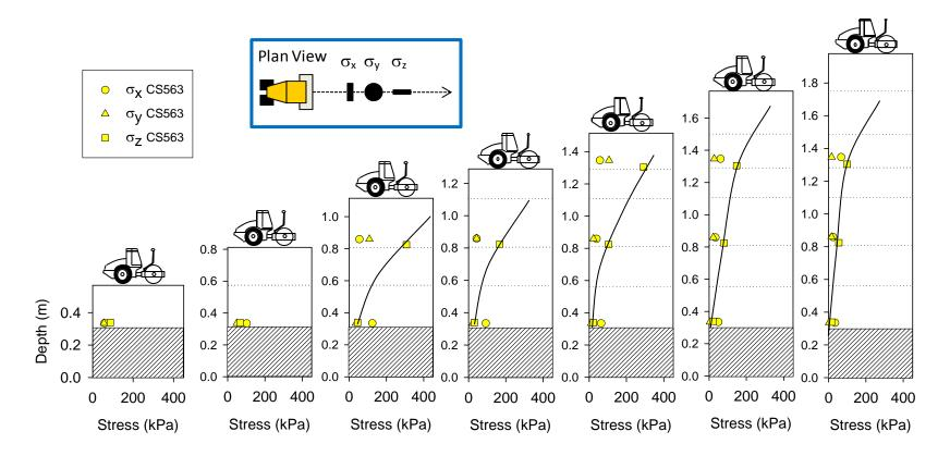
Figure 80. Stress distribution under the roller at a = 0.85 mm – TB 2
