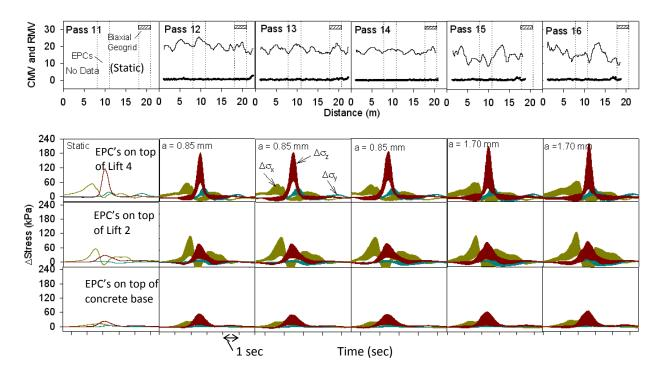
Figure 57. CMV and in-ground stress measurements for CS 683 roller passes – lift 7
