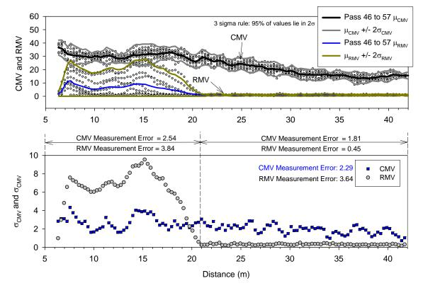
Figure 39. Repeatability analysis for CS 563 CMV/RMV measurement values at a = 1.70 mm and v = 4.8 km/h (nominal)
