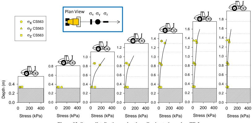
Figure 82. Stress distribution under the roller in static mode – TB 2
