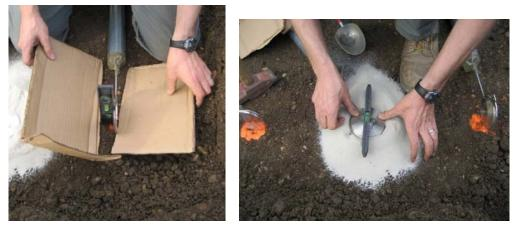
Figure 14. Leveling of EPC's and placement of thin layer of silica sand below EPC's
