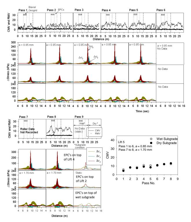
Figure 74. CMV and in-ground stress measurements for CS 563 roller passes - lift 5
