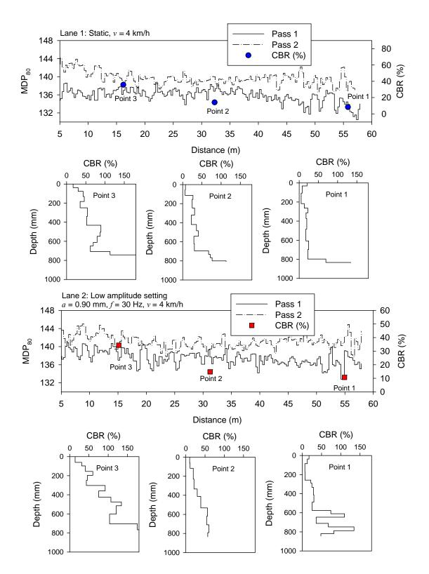
Figure 12. Comparison between MDP<sub>80</sub> and DCP-CBR point measurements –TB1 subgrade clay material (note: passes 1 and 2 with opposite machine direction of travel)
