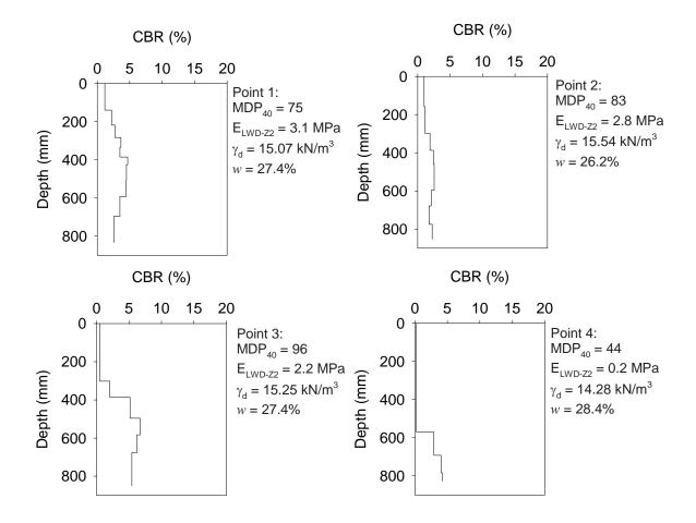
Figure 47. CBR profiles (from DCP tests) at point measurement locations – TB5 wet organic clay
