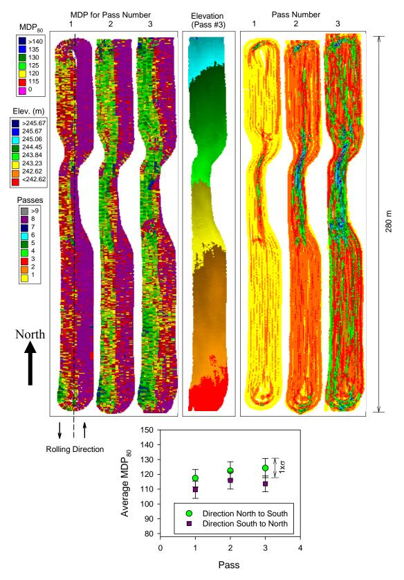
Figure 36. MDP<sub>80</sub>, elevation, pass coverage, and average MDP<sub>80</sub> (a = 0.90 mm, f = 33 Hz, v = 4 km/h) per pass on TB3 foundation subgrade layer
