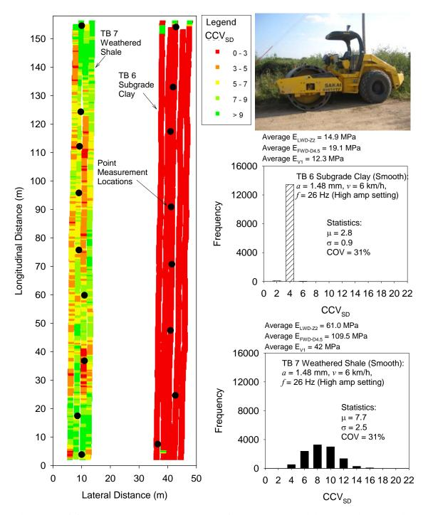
Figure 53. CCV<sub>SD</sub> map and histogram plots for TBs 6 and 7 (high amplitude setting)
