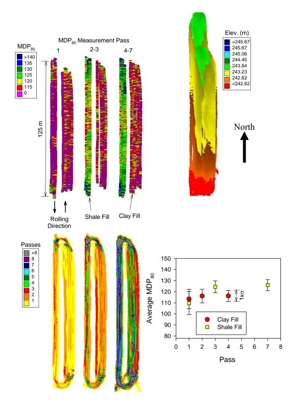
Figure 38. MDP<sub>80</sub>, elevation, pass coverage, and average MDP<sub>80</sub> (a = 0.90 mm, f = 33 Hz, v = 4 km/h) per pass on TB3 lift 2 clay fill and shale fill material
