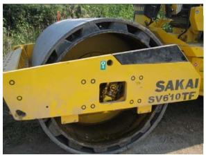
Smooth drum shell kit installed on a padfoot drum
