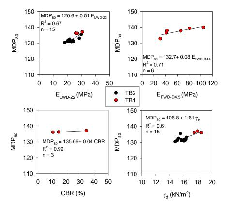
Figure 62. Regression relationships between  $MDP_{80}$  (a = 0.90 mm, f = 33 Hz, driving uphill)and in-situ point measurement values – TBs 1 and 2 subgrade clay
