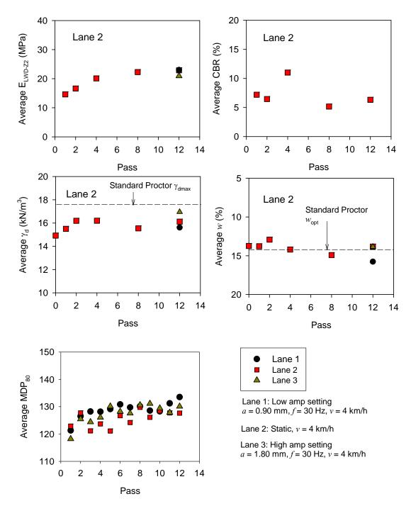
Figure 22. Comparison between average in-situ point measurement and average MDP<sub>80</sub> per pass compaction growth on TB2 subgrade clay material
