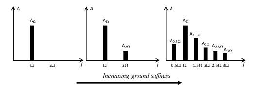
Figure 1. Changes in amplitude spectrum with increasing ground stiffness (modified from Sakai Manual)
