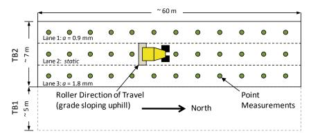
Figure 16. Experimental testing setup on TB2 (TB1 shown for reference)
