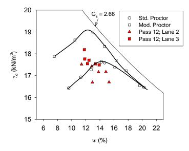
Figure 30. Comparison between laboratory  $w-\gamma_d$  relationship and in-situ  $w-\gamma_d$  point measurements after final pass on lanes 2 and 3 – TB 4 subgrade clay (USCS: CL)
