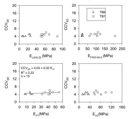
Figure 59. Regression relationships between  $CCV_{SD}$  and in-situ point measurement values from TBs 6 and 7 (a = 0.63 mm, f = 33 Hz)
