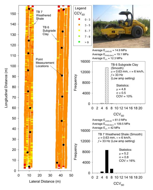
Figure 52. CCV<sub>SD</sub> map and histogram plots for TBs 6 and 7 (low amplitude setting)
