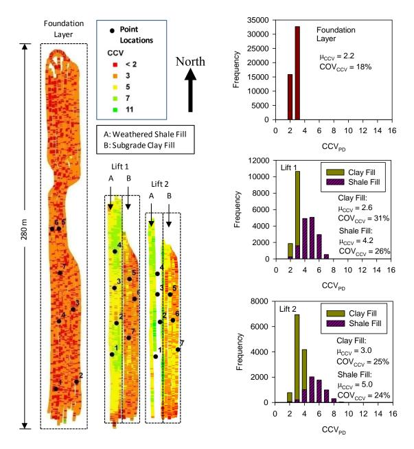
Figure 40. CCV<sub>PD</sub> maps on foundation layer and lifts 1 to 2 (a = 0.93 mm, f = 33 Hz, and v = 4 km/h)
