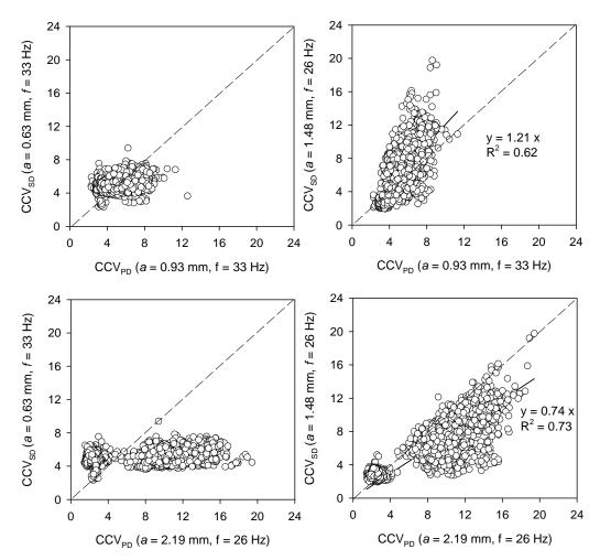
Figure 54. Regression relationships between  $CCV_{SD}$  and  $CCV_{PD}$  measurement values from TBs 6 and 7
