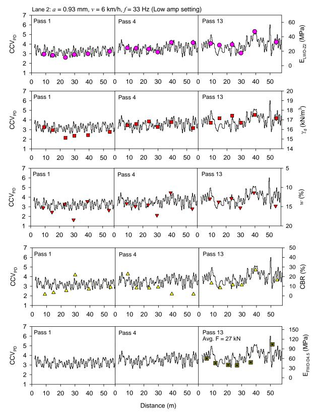
Figure 27. Comparison between CCV and in-situ point measurements – TB4 lane 2 subgrade clay material (USCS: CL)
