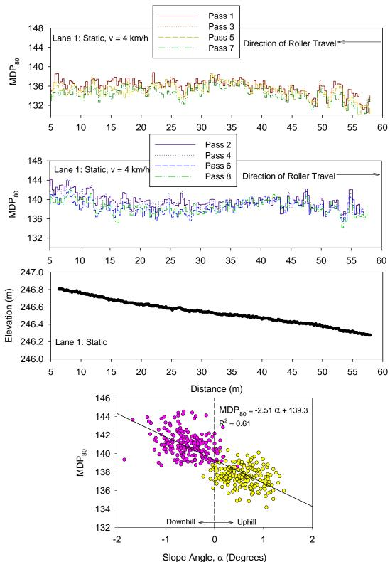
Figure 8. MDP<sub>80</sub> for multiple roller passes on TB1 subgrade clay material lane 1 and linear regression relationship between slope angle and MDP<sub>80</sub>
