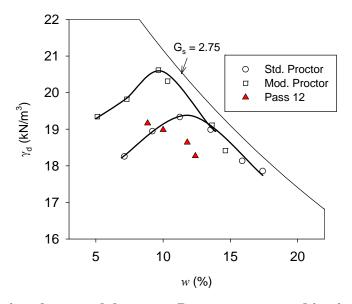
Figure 34. Comparison between laboratory Proctor curves and in-situ moisture-dry unit weight point measurements after pass 12 on TB3 lift 4 weathered shale fill material
