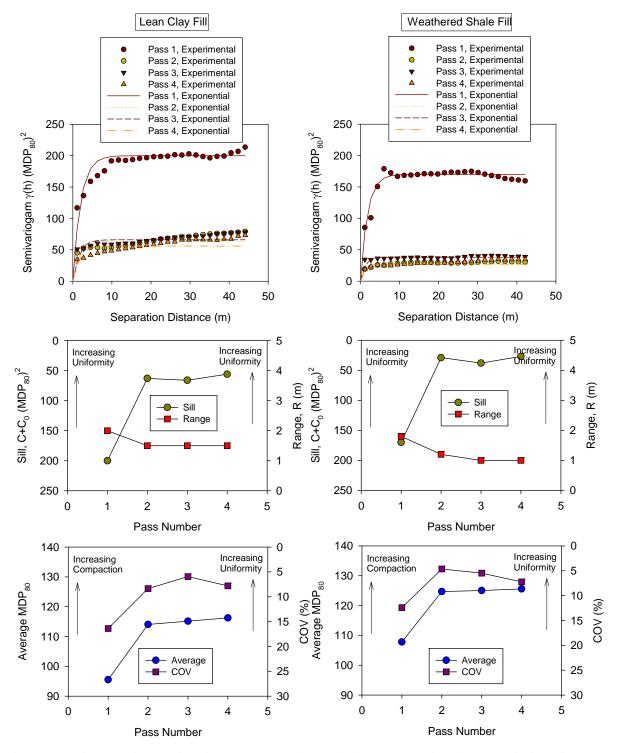
Figure 44. Change in semivariograms, spatial statistics, and univariate statistics of MDP<sub>80</sub> with pass on TB3 – lift 3 lean clay and weathered shale fill materials
