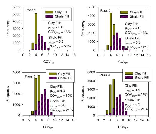
Figure 42. Histogram plots of CCV<sub>PD</sub> measurement values on lift 6 clay and weathered shale fill materials for passes 1 to 4
