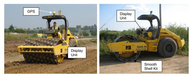
Figure 2. Sakai SV610 roller with padfoot and smooth drum setup used on the project
