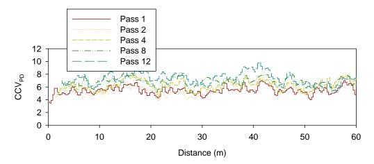
Figure 31. CCV<sub>PD</sub> measurements from multiple passes on TB3 lift 4 weathered shale fill material (a = 2.19 mm, f = 26 Hz, v = 6 km/h)
