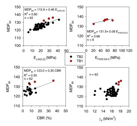
Figure 60. Regression relationships between MDP<sub>80</sub> (static – driving uphill) and in-situ point measurement values – TBs 1 and 2 subgrade clay
