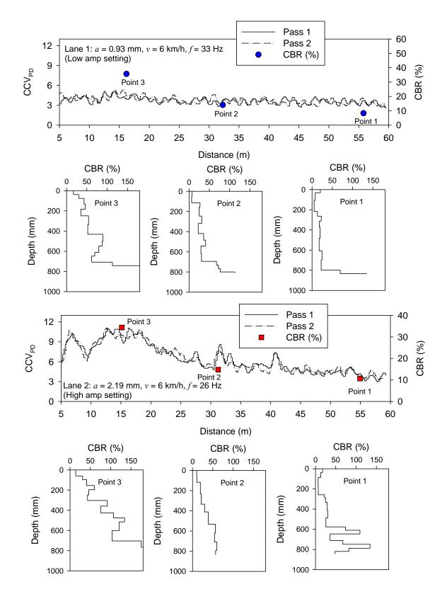
Figure 15. Comparison between CCV<sub>PD</sub> and DCP-CBR point measurements –TB1 subgrade clay material (note: passes 1 and 2 with opposite machine direction of travel)
