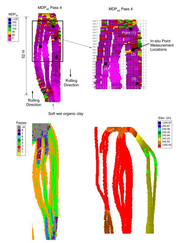
Figure 46. MDP<sub>40</sub> (static mode, v = 4 km/h) measurements on pass 4, elevation, and pass coverage information – TB5 wet organic clay
