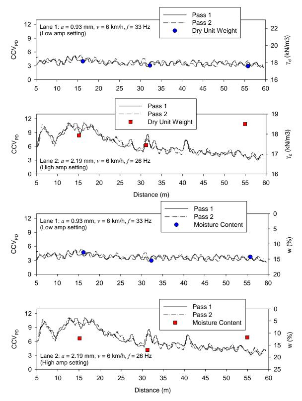
Figure 14. Comparison between CCV<sub>PD</sub> and nuclear moisture-density gauge point measurements – TB1 subgrade clay material
