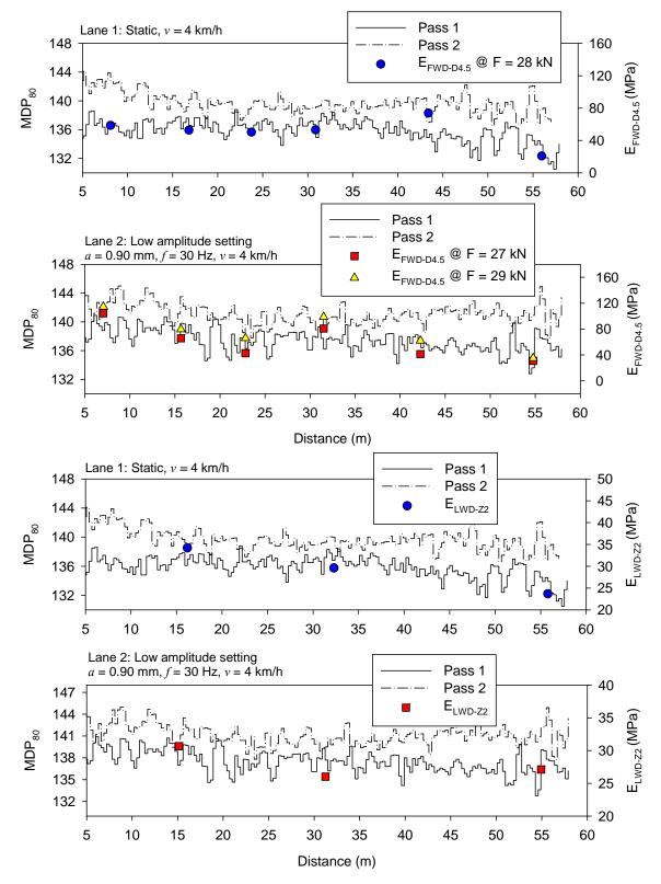
Figure 10. Comparison between  $MDP_{80}$  and  $E_{LWD-Z2}$  (top) and  $E_{FWD-D4.5}$  (bottom) point measurements – TB1 subgrade clay material (note: passes 1 and 2 with opposite machine direction of travel)
