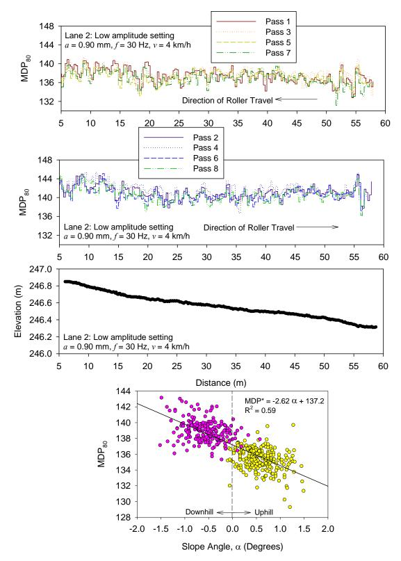
Figure 9. MDP<sub>80</sub> for multiple roller passes on TB1 subgrade clay material lane 2 and linear regression relationship between slope angle and MDP<sub>80</sub>
