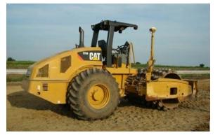
Caterpillar CS56 padfoot roller used for compaction
