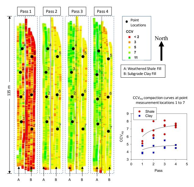
Figure 41. CCV<sub>PD</sub> maps lift 4 for passes 1 to 4 and CCV<sub>PD</sub> compaction curves at point measurement locations (a = 0.93 mm, f = 33 Hz, and v = 4 km/h)
