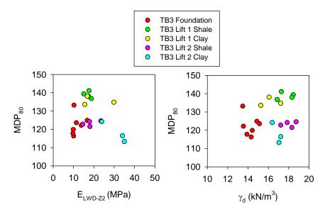
Figure 63. Regression relationships between MDP<sub>80</sub> (a = 0.90 mm, f = 33 Hz) and in-situ point measurement values – TB3 foundation layer and lifts 1 to 2
