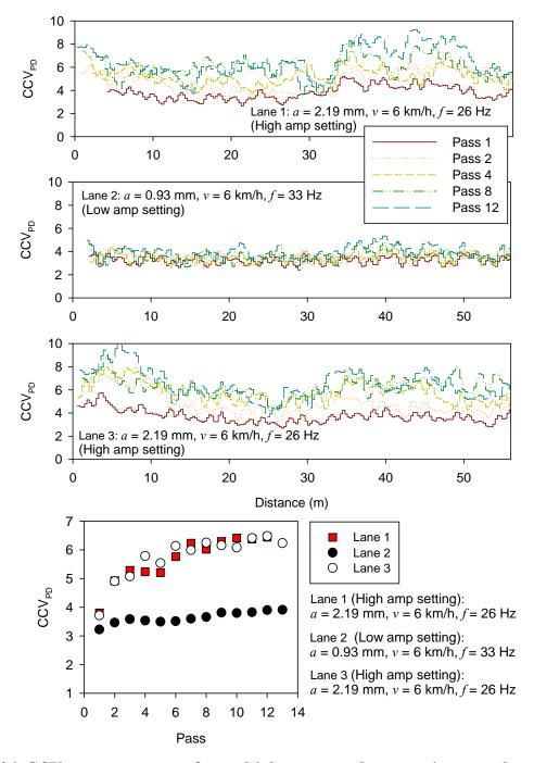
Figure 26. CCV<sub>PD</sub> measurements for multiple passes and compaction growth curves on TB4 subgrade clay material lanes 1, 2, and 3
