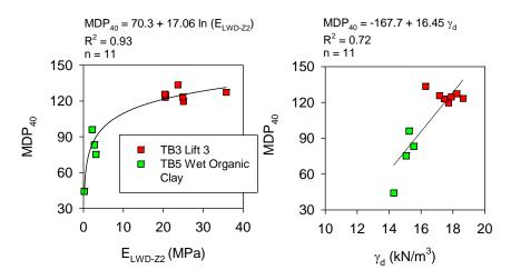
Figure 64. Regression relationships between MDP<sub>40</sub> and in-situ point measurement values – TB3 lift 3 (a = 0.90 mm, f = 33 Hz) and TB5 (static)
