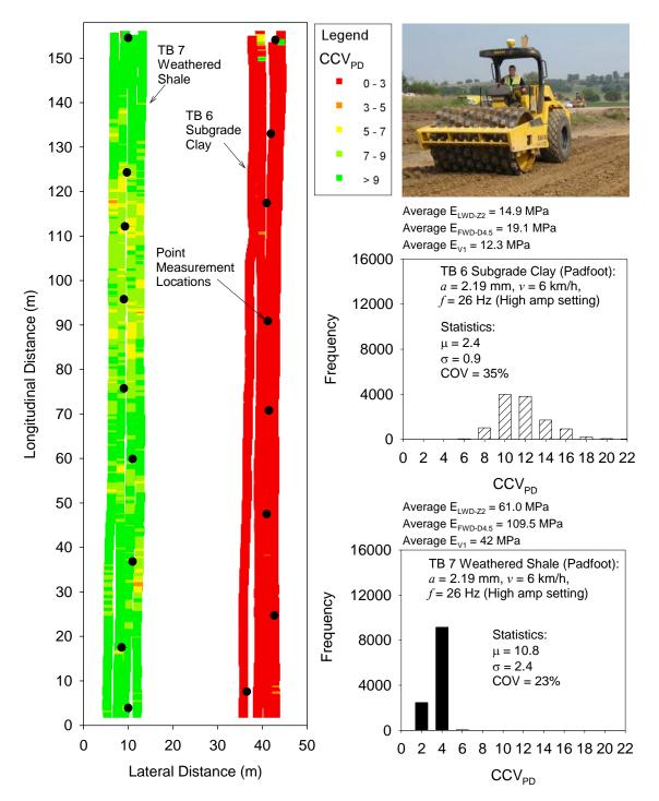
Figure 51. CCV<sub>PD</sub> map and histogram plots for TBs 6 and 7 (high amplitude setting)
