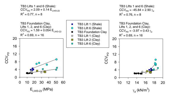
Figure 57. Regression relationships between  $CCV_{PD}$  and in-situ point measurement values from TB3 production area (a = 2.19 mm, f = 26 Hz)
