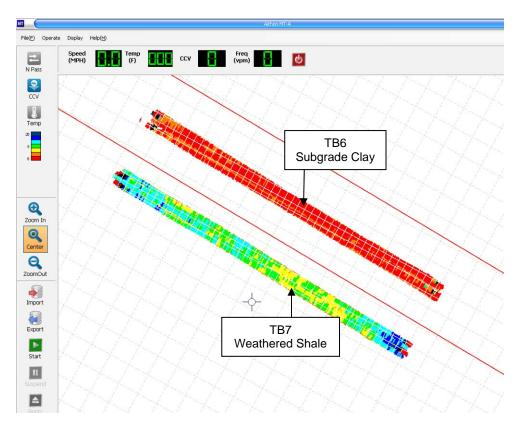
Figure 49. AithonMT display of  $CCV_{SD}$  map (a = 1.48 mm, f = 26 Hz)
