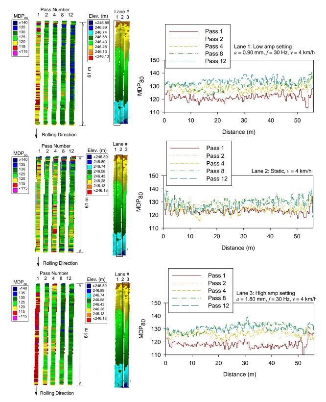
Figure 18. MDP<sub>80</sub> measurements for multiple passes on TB2 subgrade clay material lanes 1, 2, and 3
