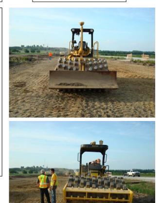
Caterpillar (top) and Sakai (bottom) padfoot rollers used on the test bed
