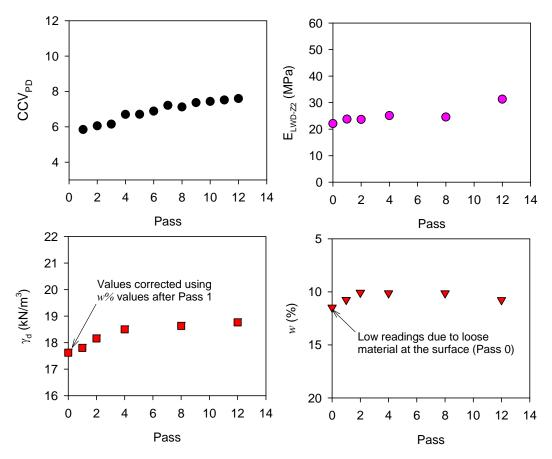
Figure 33. Comparison between average  $CCV_{PD}$  (a = 2.19 mm, f = 26 Hz, v = 6 km/h) and in-situ point measurement compaction growth per pass on TB3 lift 4 weathered shale fill material
