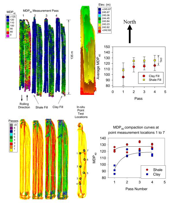
Figure 39. MDP<sub>40</sub>, elevation, pass coverage, average MDP<sub>40</sub> (a = 0.90 mm, f = 33 Hz, v = 4 km/h) per pass, and MDP<sub>40</sub> at select point locations on TB3 lift 3 clay fill and shale fill material
