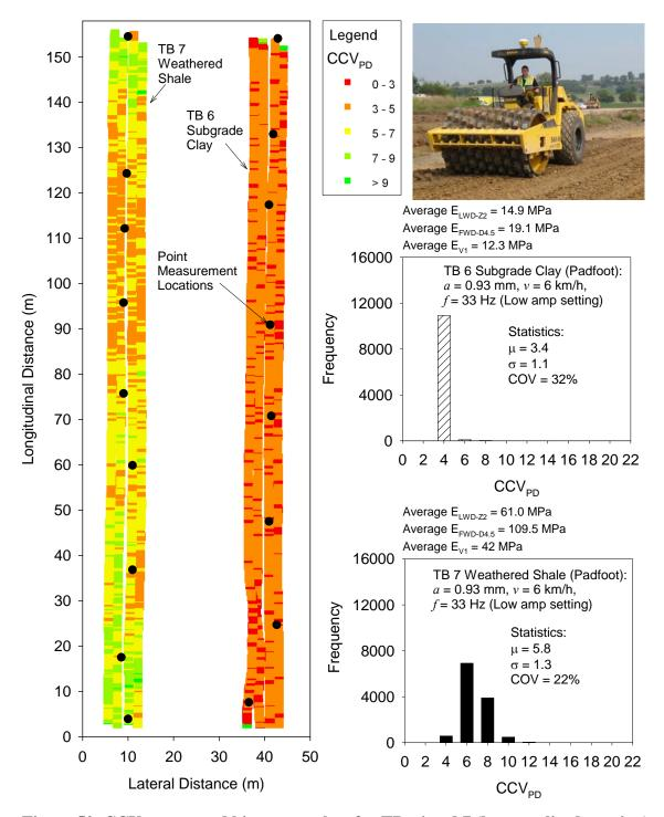
Figure 50.  $CCV_{PD}$  map and histogram plots for TBs 6 and 7 (low amplitude setting)
