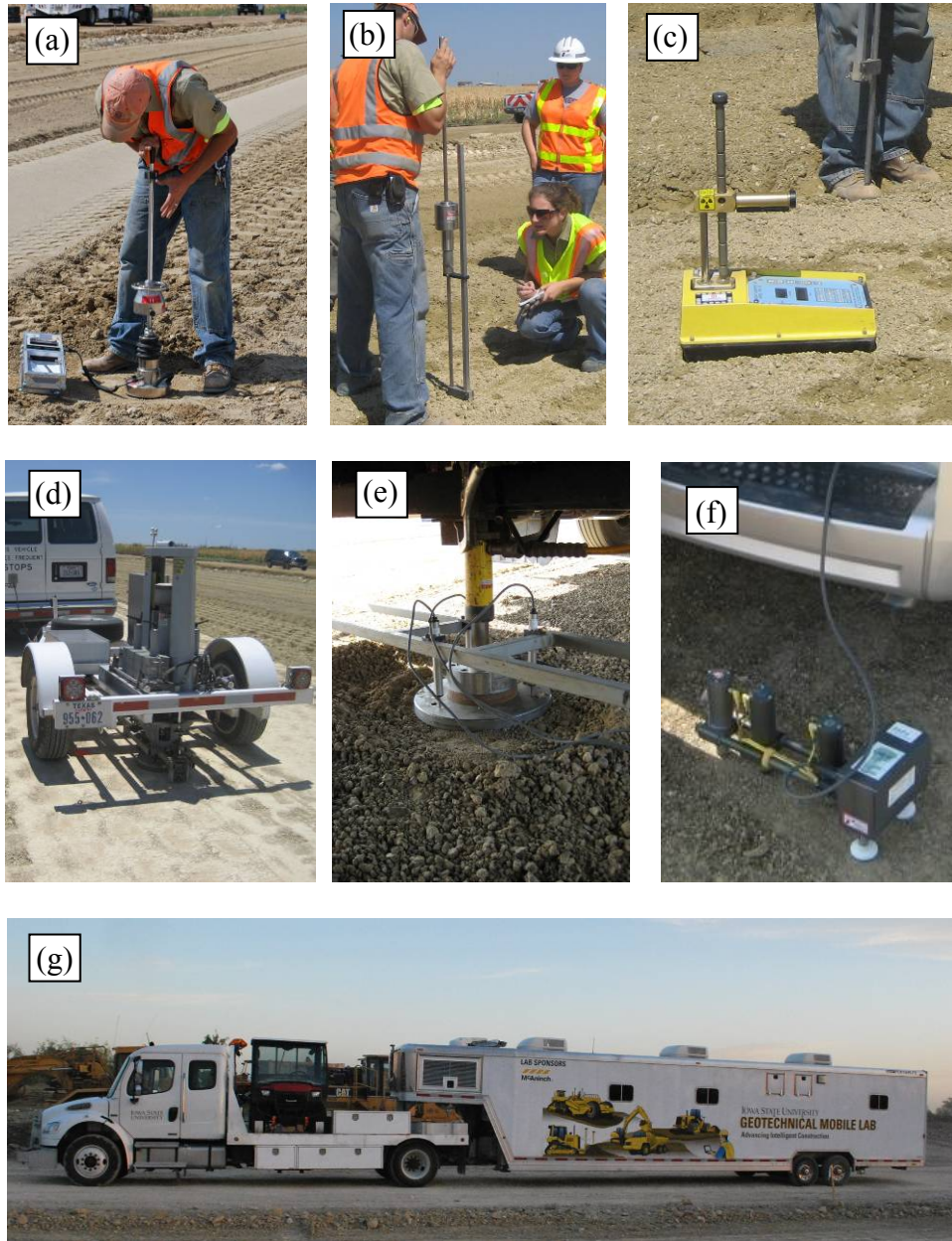
Figure 5. In-situ testing methods used on the project: (a) 200-mm diameter plate Zorn LWD, (b) dynamic cone penetrometer, (c) calibrated nuclear moisture-density gauge, (d) 300-mm diameter Dynatest FWD, (e) 300-mm diameter static PLT, (f) D-SPA, and (g) Iowa State University geotechnical mobile lab
