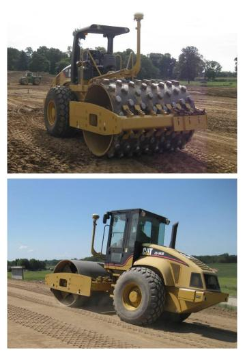
Figure 1. Caterpillar CS56 smooth drum with padfoot shell kit (top) and Caterpillar CS563E smooth drum (bottom) IC rollers used on the project
