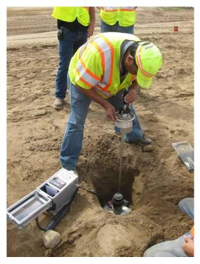
Figure 19. LWD testing at multiple depths on TB2 – Granular embankment fill
