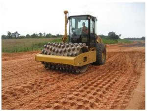
Caterpillar CP-56 roller used on the test bed
