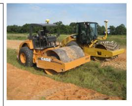
Machine Nominal settings (Section A): Caterpillar padfoot CP56: low amp - a = 0.90mm, f = 30 Hz, v = 4 km/h on lanes 1 to 3 and static, v = 4 km/h on lanes 4 to 6 Case/Ammann smooth SV212: Ecc = 15% –  $a \sim 0.9$  mm, f = 27 Hz, v = 4 km/h. Caterpillar pneumatic tire PS360C: Static. Machine Nominal settings (Section B): Caterpillar padfoot CP563: low amp. Sakai smooth SV505T: low amp. Caterpillar pneumatic tire PS360C: Static.
