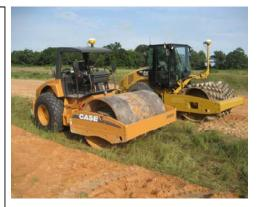
Machine Nominal settings (Section A): Caterpillar padfoot CP56: low amp - a = 0.90 mm, f = 30 Hz, v = 4 km/h. Case/Ammann smooth SV212: Ecc = 15%  $-a \sim 0.9 mm$ , f = 27 Hz, v = 4 km/h. Caterpillar pneumatic tire PS360C: Static. Machine Nominal settings (Section B): Caterpillar padfoot CP563: Static. Sakai smooth SV505T: Static. Caterpillar pneumatic tire PS360C : Static.
