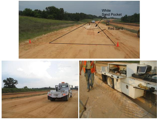
Figure 51. TB7 granular subgrade material (red sand subgrade with isolated white sand pocket)
