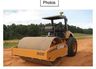
Case/Ammann roller used for mapping
