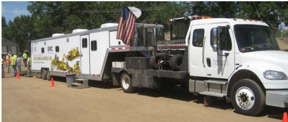
Figure 10. Iowa State University geotechnical mobile laboratory
