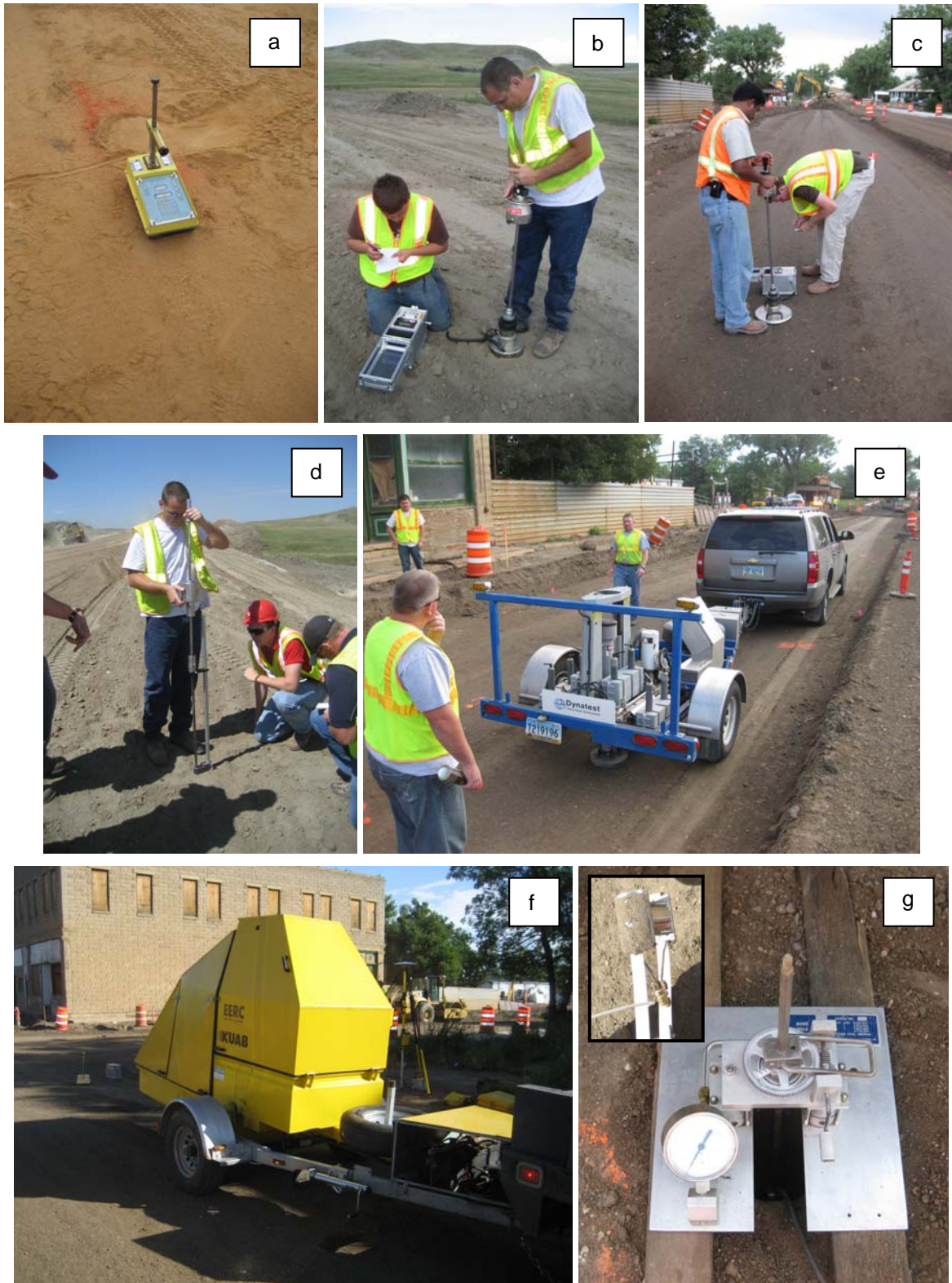
Figure 8. In-situ testing methods used on the project: (a) Humboldt nuclear gauge, (b) 200 mm Zorn LWD, (c) 300 mm Zorn LWD, (d) dynamic cone penetrometer, (e) Dynatest FWD, (f) KUAB FWD, (g) Iowa BST (expandable contact plates shown in the insert)
