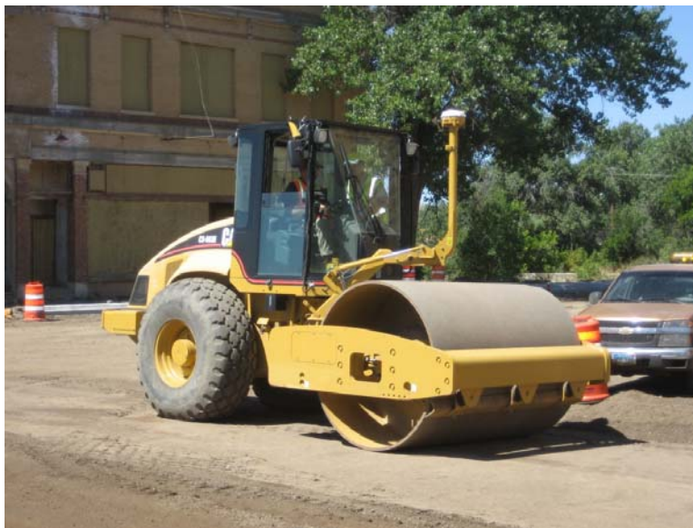
Figure 1. Caterpillar CS56 smooth drum with padfoot shell kit (top) and Caterpillar CS563E smooth drum (bottom) IC rollers used on the project
