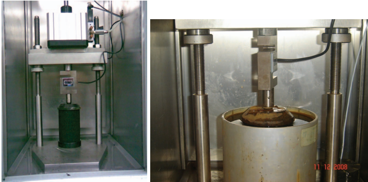
Figure 3-2. Flow number test setup
