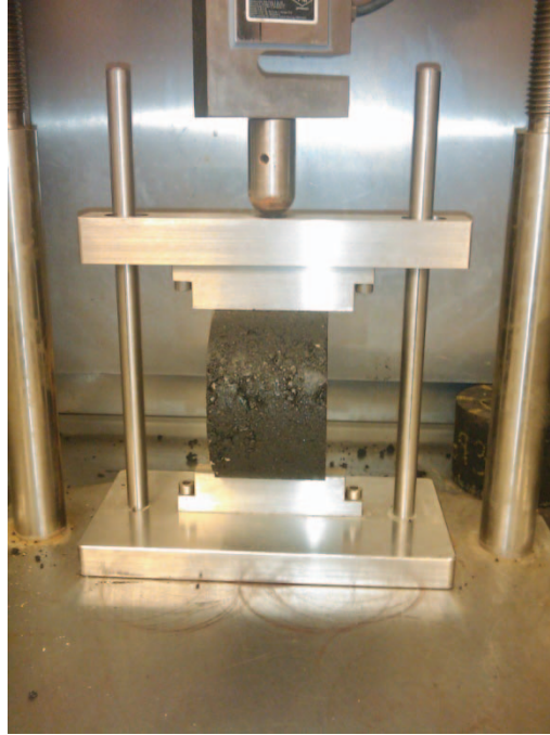
Figure 3-3. Indirect tensile strength test setup
