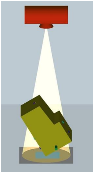
Figure 19. #4 Reinforcing steel with 50 percent corrosion loss at realistic angle
