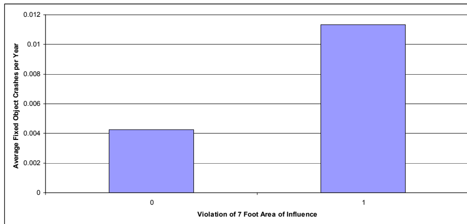
Figure 5-37. Violation of 7 ft area of influence in 15 m analysis
