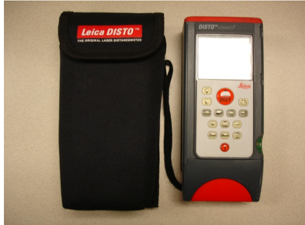
Figure 4-4. DISTO Classic 5 laser distance meter
