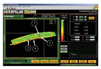
Compaction monitor showing areas of unstable subgrade (red)
