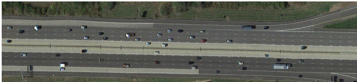
Figure 4.4. Example of add and drop lanes
