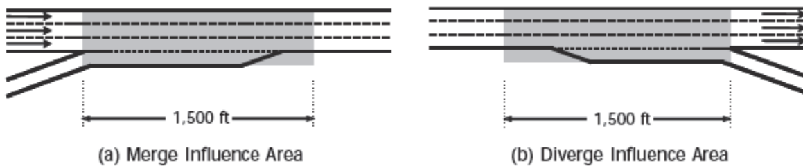
Figure 2.6. Interchange influence area (top) and merge and diverge influence areas (bottom)
