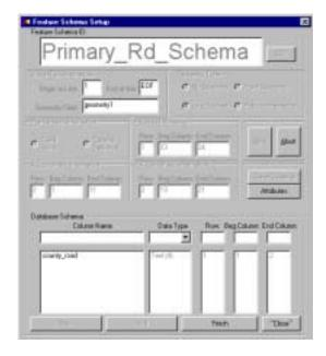
Repeat the above process to add a column called 'Route' having a length of 6 characters. The row number for the route data is 1, and the positions range from 16 to 19. After clicking the *Add* button to add the final column, click the *Finish* button to complete the Database Schema.
