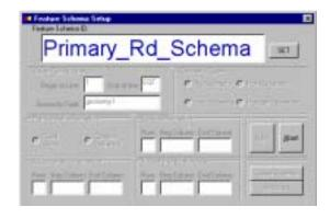
**Step 2.** Select the type of geometry the schema file will define. Click the *Line Geometry* option button in the Geometry Type box. Doing so will cause the appropriate textboxes needed for inputting line Geometry Schema information to enable.
