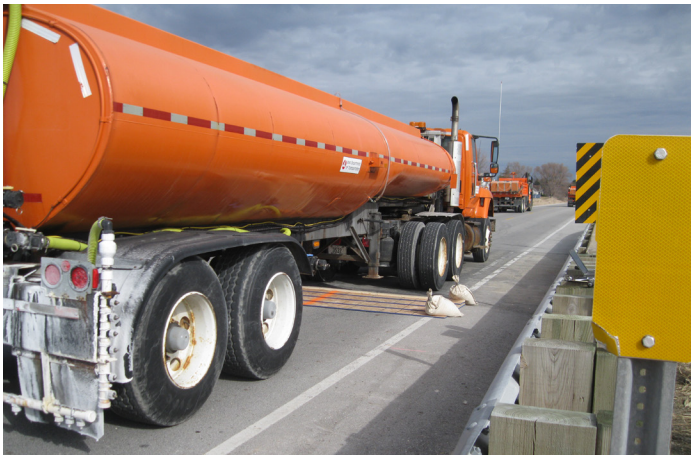
Semi-truck crossing the instrumented slab bridge with Level 2 entrance conditions (fabricated ramp at the approach joint)
