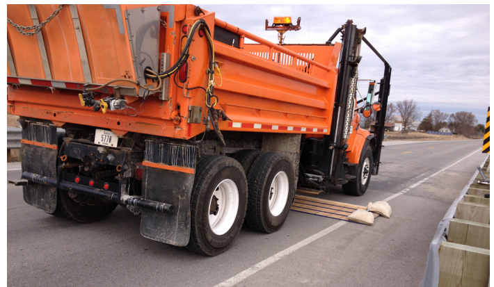
Empty dump truck crossing the instrumented slab bridge with Level 1 entrance conditions (fabricated ramp 10 ft from joint)
