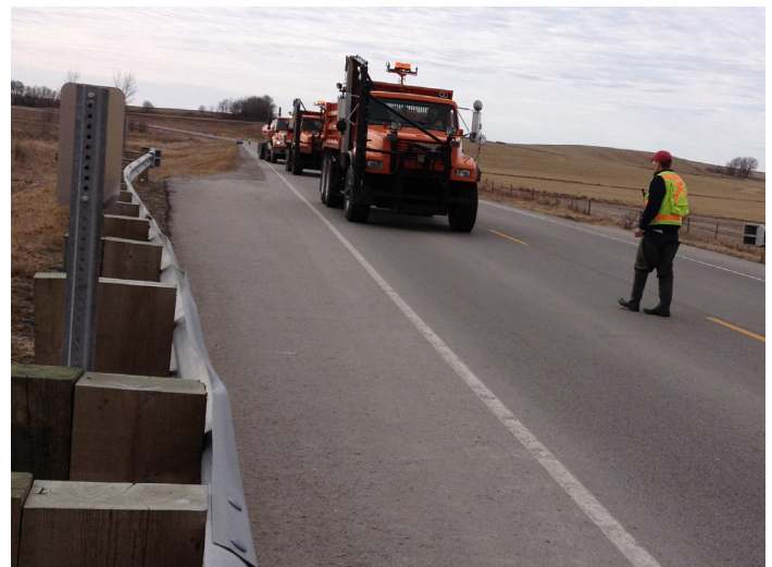
Empty dump truck crossing the instrumented slab bridge with As-is entrance conditions during load testing
