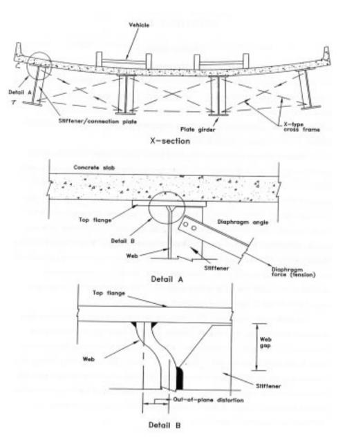
This figure represents out-of-plane girder web distortion in the gap region.
