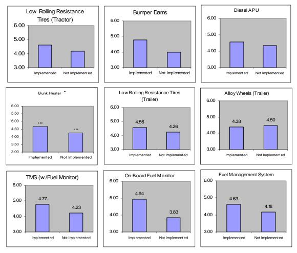
Figure 10. Fuel performance comparison (implemented vs. non-implemented)
