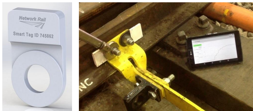
Figure 2-17. Smart washer and data reading unit
