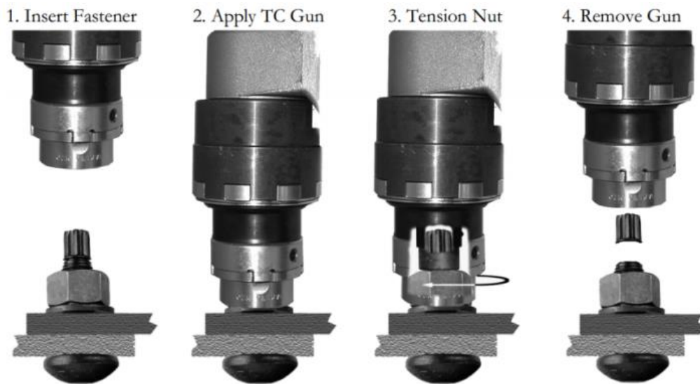
Figure 2-10. Twist-off-type installation procedure
