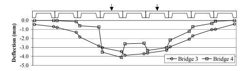
FIGURE 5. Transverse Centerline Deflections: Center Lane Loading
