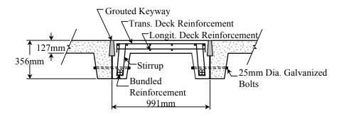
FIGURE 2. Type I PCB Panel Cross-Section
