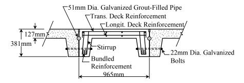
FIGURE 3. Type II PCB Panel Cross-Section
