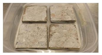
Samples partially immersed in testing solution
