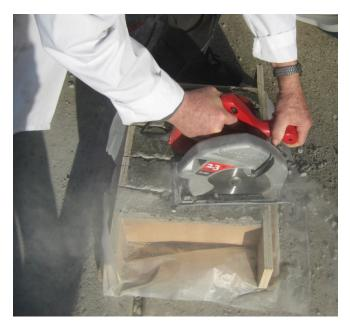
Saw cutting a test slab using poor practices
