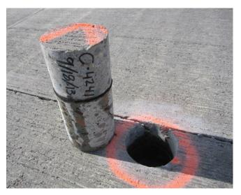
Sample core retrieved in 2013 showing the relationship to Joint 4241 Cell 505 with its fabric bond-breaker
