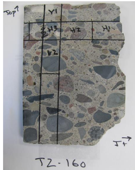
Figure 7. Slab marked for cutting into billets, showing billet orientations
