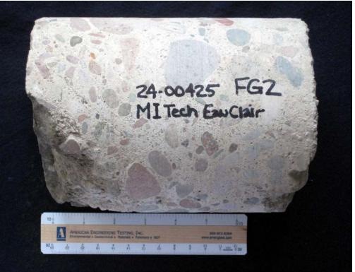
SAMPLE ID: FG2 **DESCRIPTION:** Core sample taken directly through a joint as received. Top surface is left.
