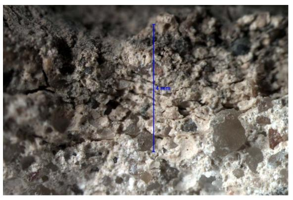
SAMPLE ID: FG1 DESCRIPTION: Highly concentrated anastomosing microcracking in carbonated paste directly adjacent to distressed joint plane (top of image); in freshly fractured cross sectional surface of core. 15x
