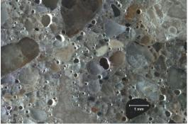
Magnification: 15x Description: Air void system- top 10mm of core.
