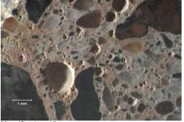
Magnification: 15x Description: Hardened air void system 150mm from the top surface and at the joint crack.
