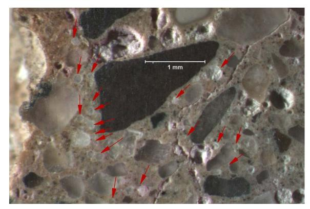
SAMPLE ID: DESCRIPTION: The great majority of fine spherical entrained air voidspaces at 98mm depth in the core and directly D adjacent to the distressed joint (left) are filled with secondary ettringite.
