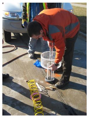
Figure 5. Inserting the device into a core hole
