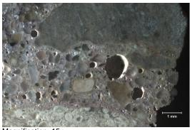
Magnification: 15x Description: Air void system at joint 140mm depth.
