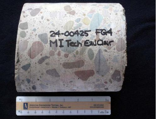
SAMPLE ID: FG4 **DESCRIPTION:** Core sample as received. Top surface is left.
