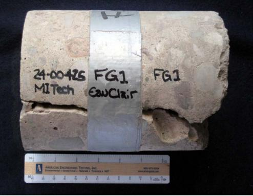
SAMPLE ID: FG1 DESCRIPTION: Core sample taken directly through a joint as received. Top surface is left.
