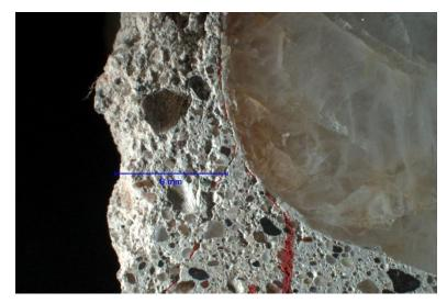
Figure 3. Cracks concentrated adjacent to the coarse aggregate in FG1
