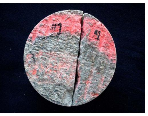
**SAMPLE ID:** #1 **DESCRIPTION:** Top surface of the core sample, taken directly through a joint, as received.
