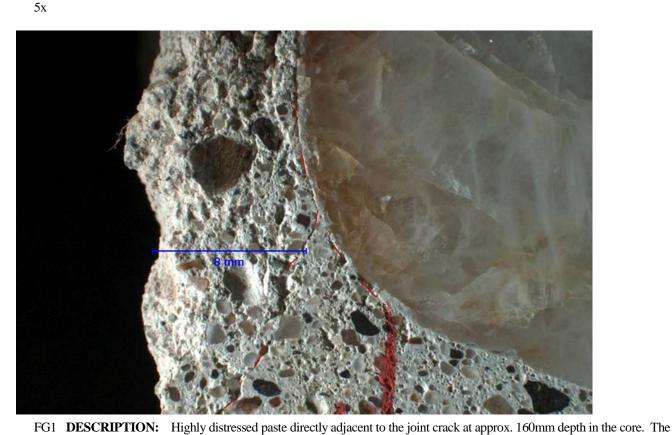
paste is lighter colored, softer, and filled with concentrated fine microcracking.
