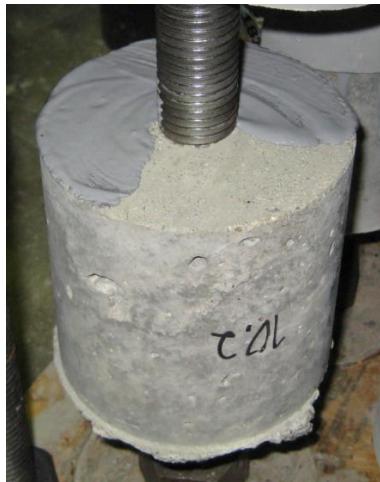
Figure 3.8. Epoxy-bonded test specimen
