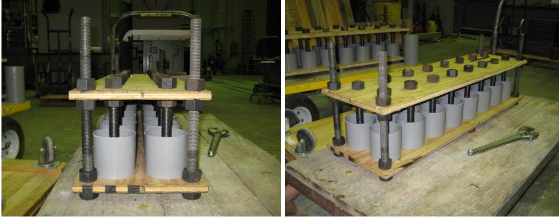
Figure 3.3. Direct tension test precast concrete half-specimen jig
