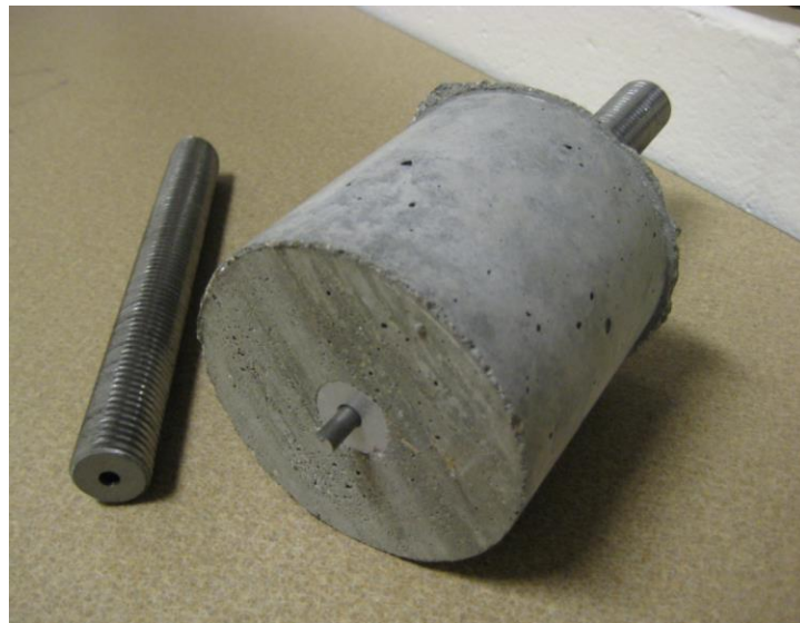
Figure 3.2. Direct tension test half-specimen connection
