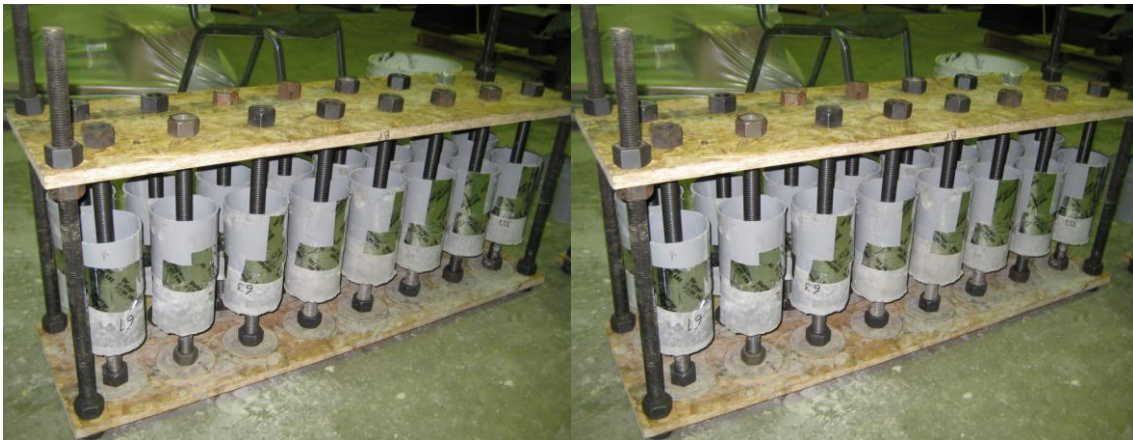
Figure 3.4. Direct tension test UHPC half-specimen jig
