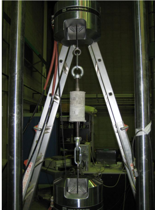
Figure 3.5. Direct tension setup
