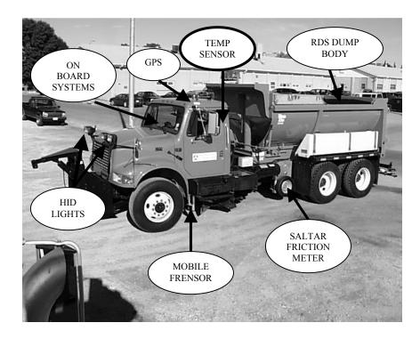
FIGURE 1: Phase IV Highway Maintenance Concept Vehicle (2001-2002)
