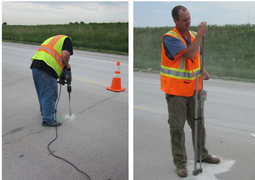
Figure 16. Dynamic cone penetrometer test
