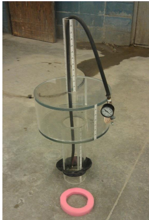
Figure 17. Core hole permeameter (CHP) device and components.
