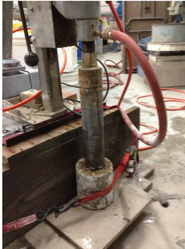
Figure 8. Picture of coring 3 in. cores from field 6 in. cores
