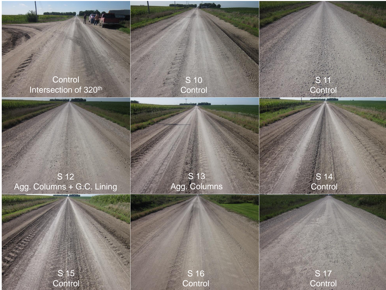
Figure 129. (continued). Survey photos of Vail Avenue demonstration sections (September 2, 2014)
