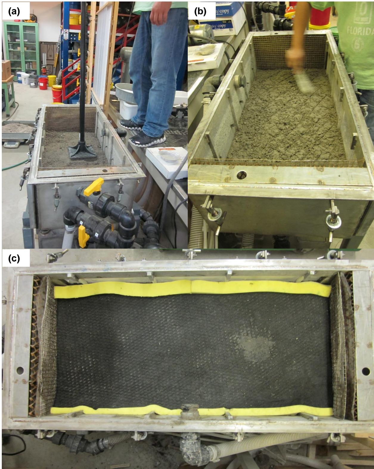
Figure 120. HPT specimen compaction: (a) compact specimen in several lifts, (b) scarify surface after each compaction lift, and (c) place geocomposite at middle of specimen and seal gaps between geocomposite and soil tank using closed-cell foam
