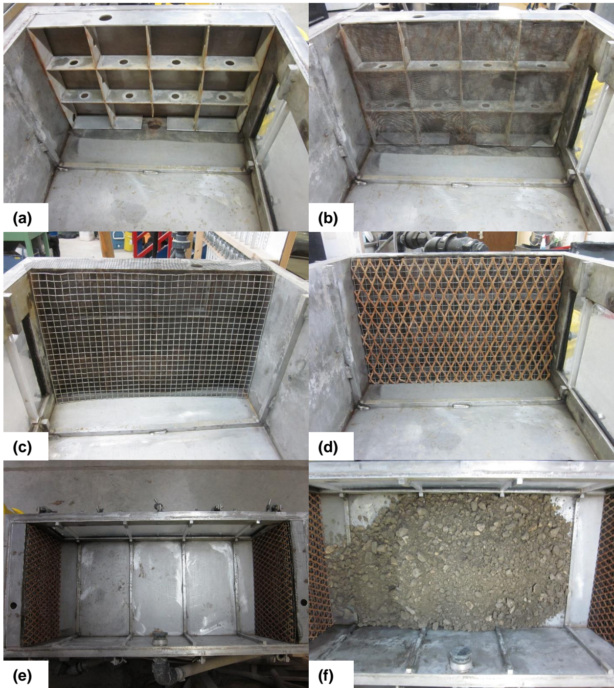
Figure 119. HPT soil tank set up: (a) place fine screen and screen support on top of inlet and outlet, (b, c, d, and e) place three screens with different opening sizes next to the screen support, (e) place specimen material in soil tank
