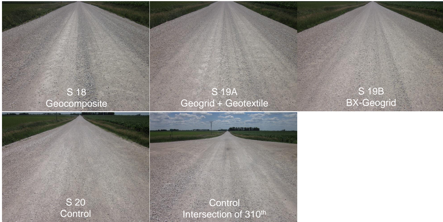
Figure 128. (continued). Survey photos of Vail Avenue demonstration sections (July 3, 2014)
