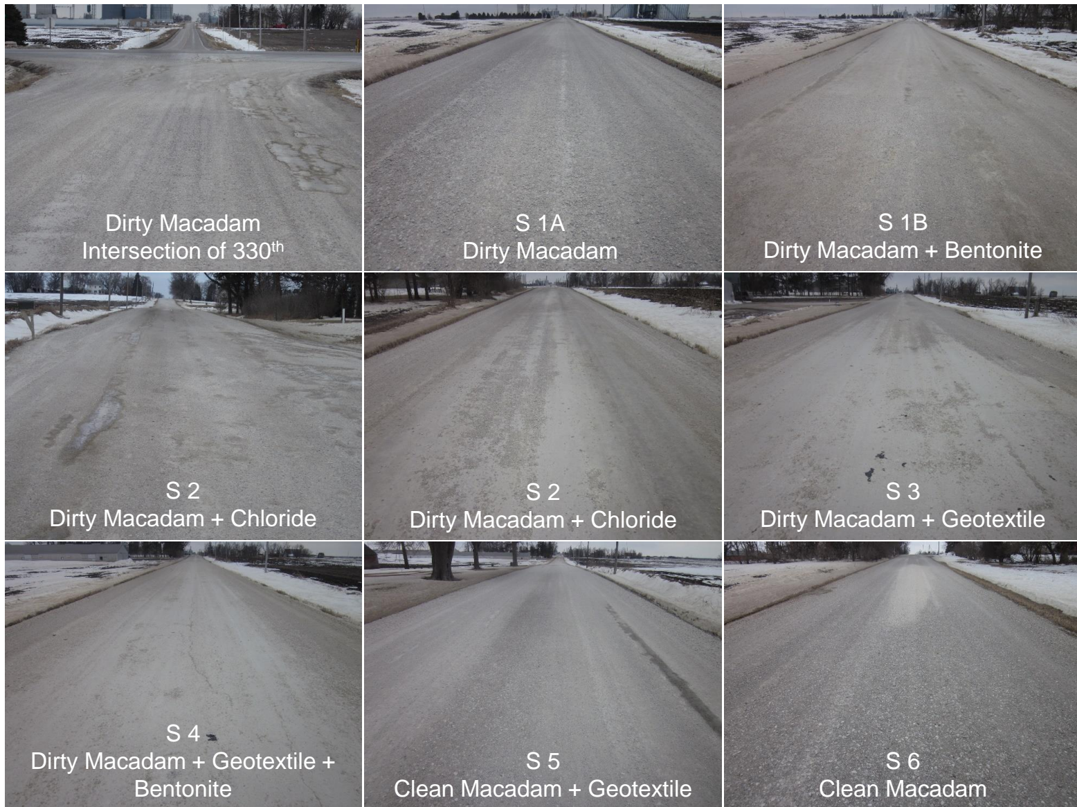
Figure 131. Survey photos of Vail Avenue demonstration sections (February 24, 2015)
