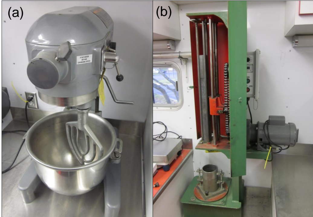
Figure 5. (a) Hobart mixer and (b) automated mechanical rammer used in this study
