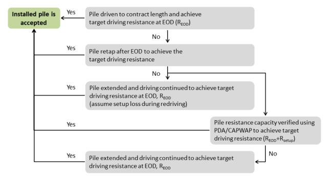
Figure 2.2. Construction control flow chart for friction piles embedded in cohesive soil and retap performed after EOD
