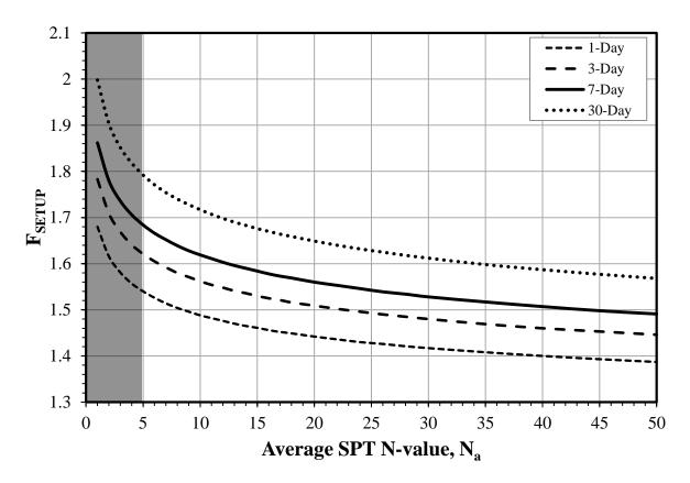
Figure D.1. Pile setup factor chart for WEAP as a construction control method
