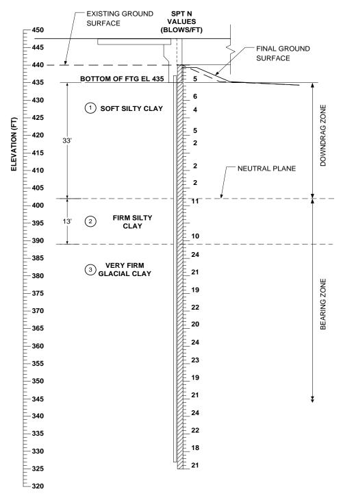
Figure 3.10. Track 1 Example 3: Soil profile
