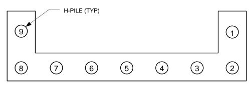
Figure 5.2. Track 3 Example 1: Pile arrangement at an abutment
