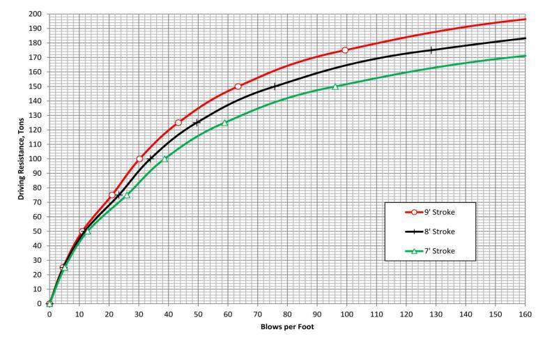
Figure 5.7. Track 3 Example 2: WEAP bearing graph for the west abutment
