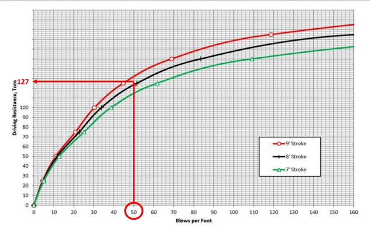
Figure 3.6. Track 1 Example 1: WEAP bearing graph for west abutment piles
