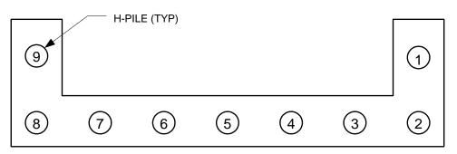
Figure 3.15. Track 1 Example 5: Pile arrangement at an abutment
