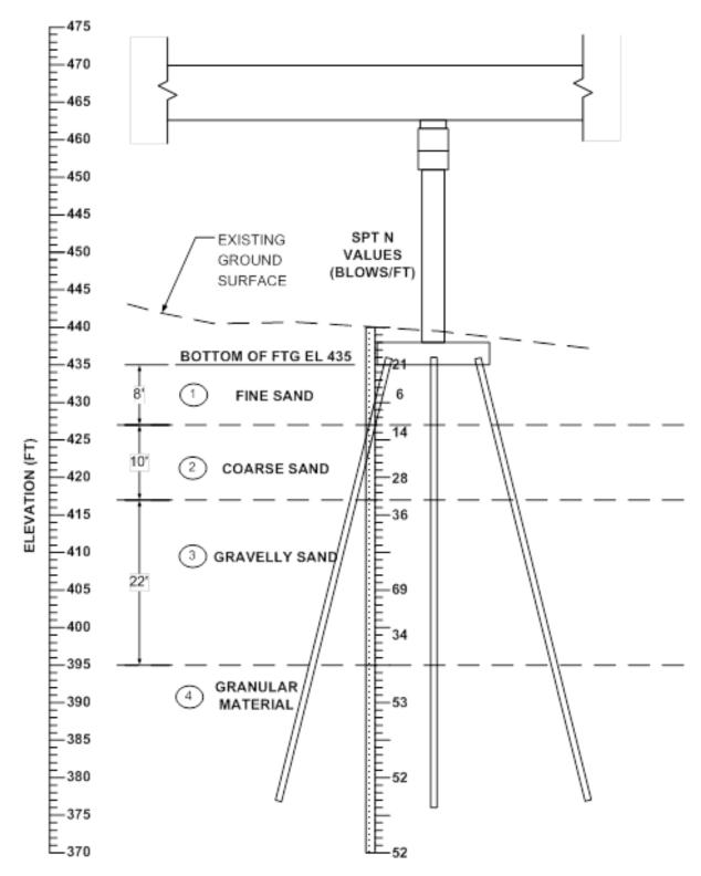
Figure 3.13. Track 1 Example 4: Soil profile
