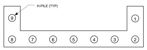
Figure 4.2. Track 2 Example 1: Pile arrangement at an abutment
