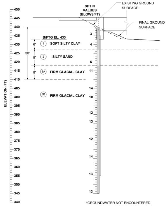
Figure 4.1. Track 2 Example 1: Soil profile
