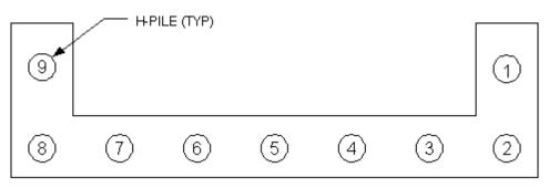
Figure 3.2. Track 1 Example 1: Pile arrangement at an abutment
