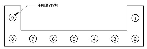
Figure 5.5. Track 3 Example 2: Pile arrangement at an abutment
