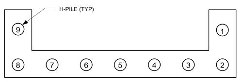
Figure 3.11. Track 1 Example 3: Pile arrangement at an abutment
