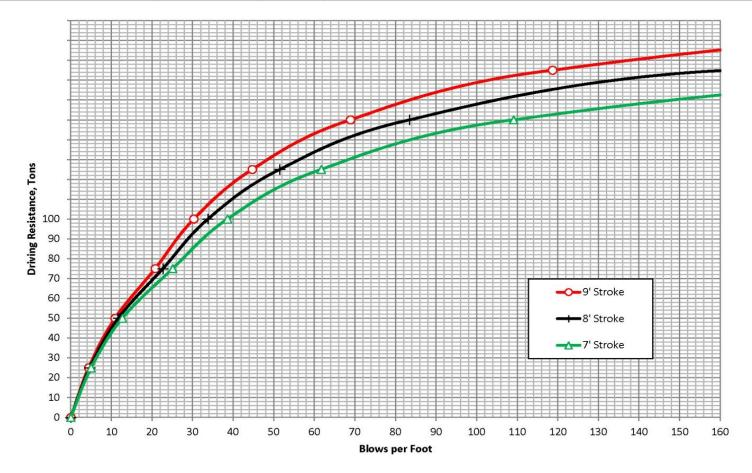
Figure 3.5. Track 1 Example 1: General WEAP bearing graph
