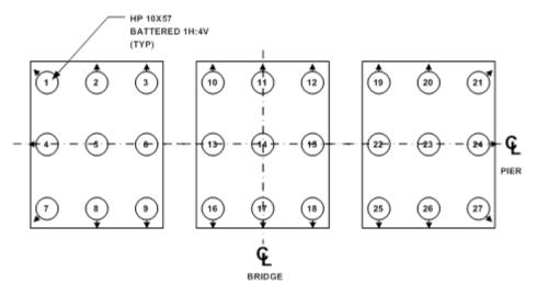
Figure 3.14. Track 1 Example 4: Pile arrangement at pile piers
