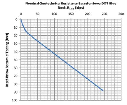
Figure 3.3. Track 1 Example 1: Plot of nominal geotechnical resistance versus depth
