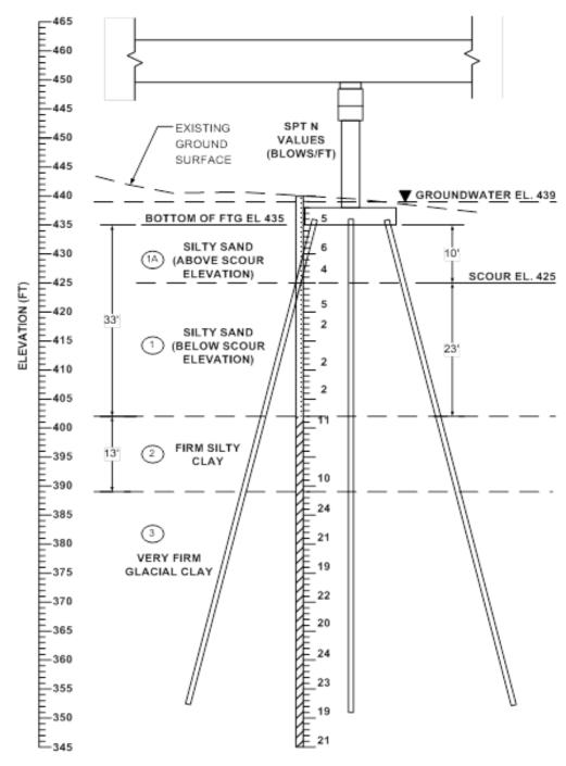
Figure 3.8. Track 1 Example 2: Soil profile
