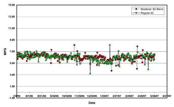
Figure 4. Daily mileage data comparisons for trucks using B0 and B2
