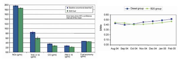
Figure 3. Data on emissions and average maintenance costs for using B0 and B20 from a Denver bus study project
