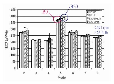
Figure 1. Engine brake specific fuel consumption data for a specific commercial diesel engine
