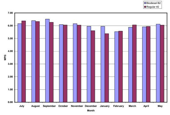
Figure 5. Monthly mileage data comparisons for trucks using B0 and B2
