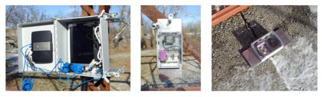
Figure 8. Attachment of the data acquisition system (left), attachment of sensor to a tension tie (middle), and placement of sensor on the deck (right) during field implementation test
