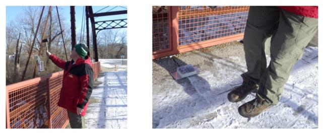
Figure 9. Impact on a tension tie via rubber mallet (left) and impact on the deck by jumping (right) during field implementation testing
