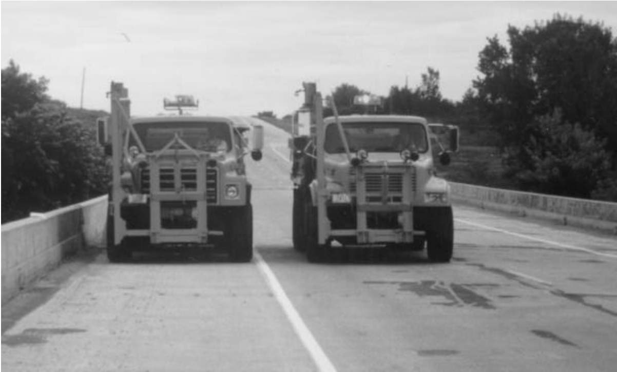
Figure 7. Trucks used for testing Bridge X1
