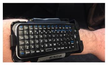
Figure 3. Arm-mounted wireless mini keyboard for dynamic simulation control
