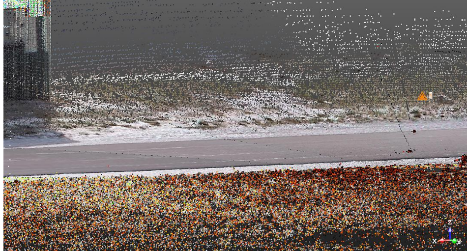
Figure 3. Registered point cloud of a new asphalt pavement surface
