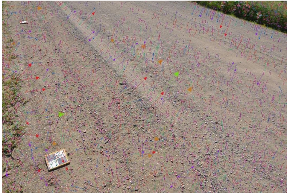
Figure 4. SFM key point recognition using a difference-of-Gaussian function (see colored arrows)
