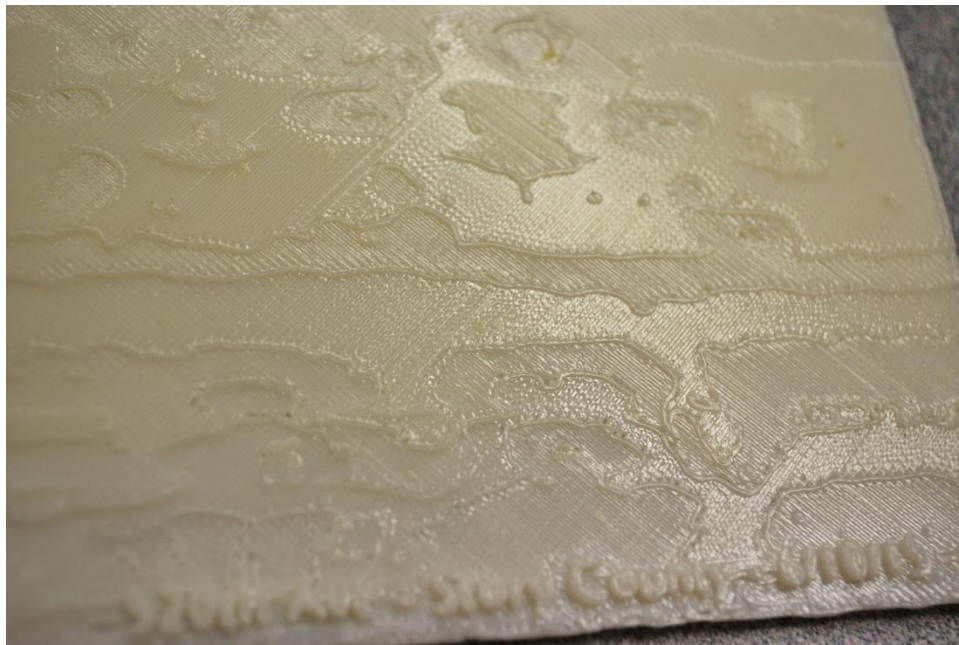
Figure 9. 3D-printed model of gravel road from a low-resolution Stratasys Mojo printer
