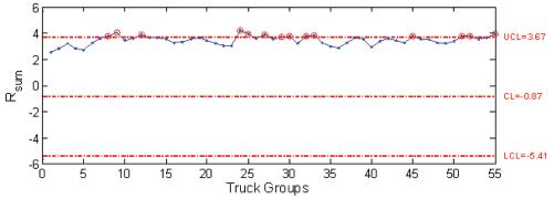
Sample control chart indicating damage detection (red-circled data points above the upper control limit (UCL)
