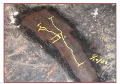
Top of bottom web plate cracking
