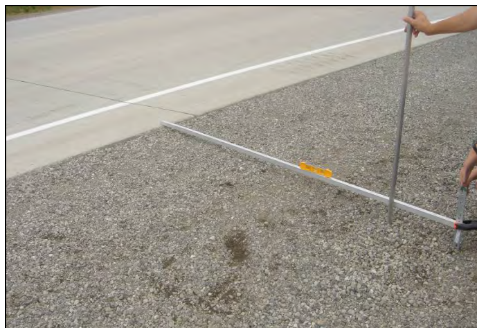
Figure 136. Determining shoulder elevations relative to the pavement, September 22, 2005
