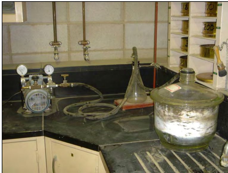
Figure 144. Vacuum saturation apparatus
