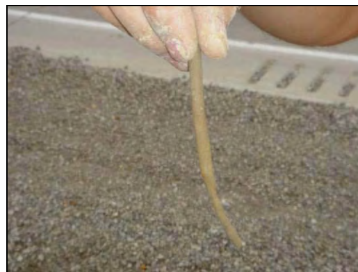
(b) Clay material rolled into thin thread
