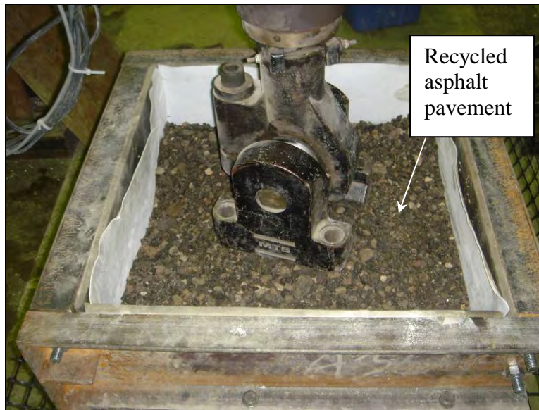
Figure 213. RAP material overlying soft subgrade soil
