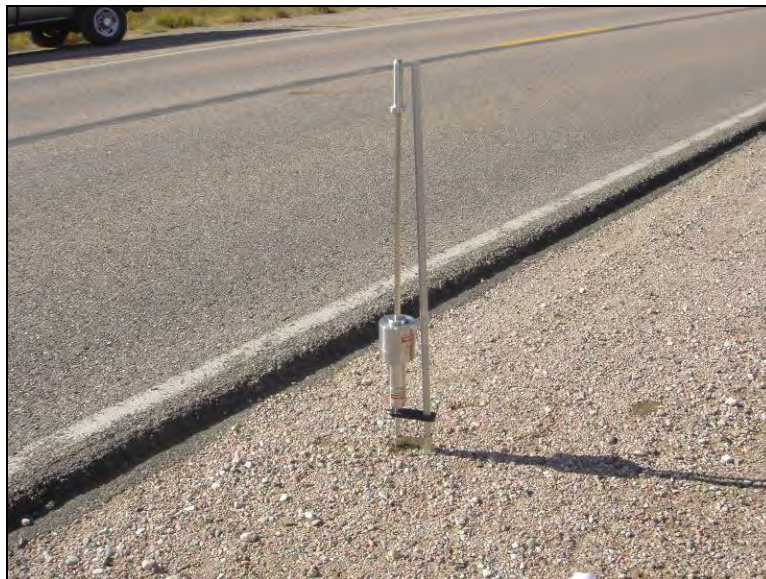
Figure 61. Performing DCP test at the westbound shoulder, October 14, 2005
