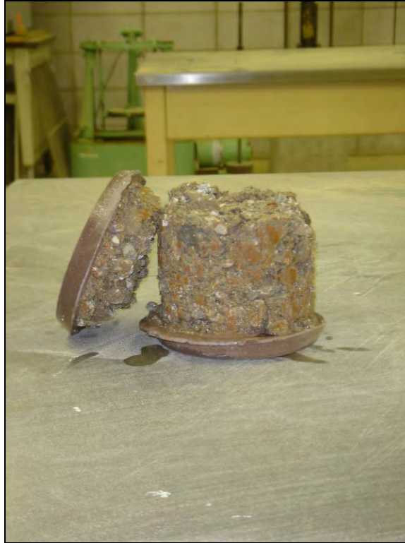
Figure 94. Disintegrated specimen after soaking for four hours
