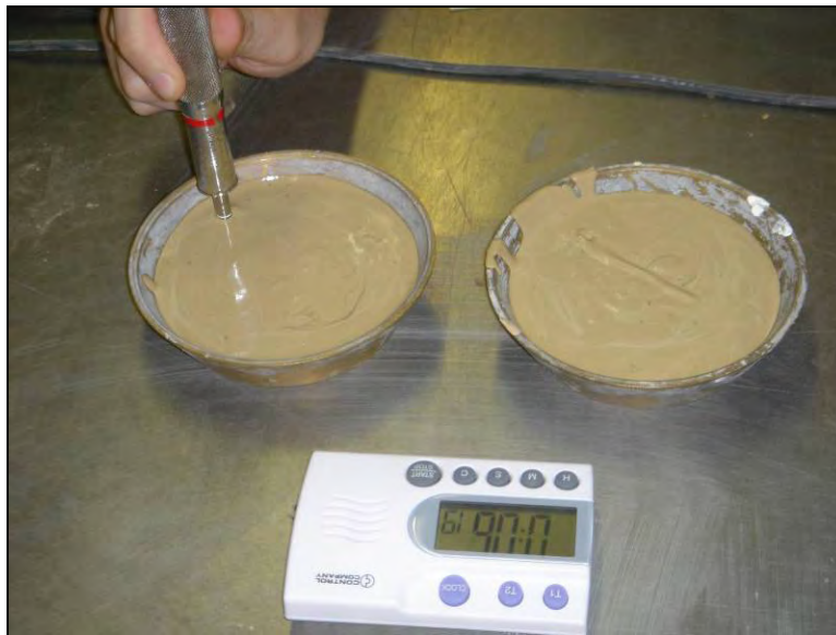
Figure 142. Fly ash set time testing
