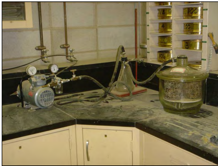
Figure 104. Vacuum saturation test conducted on granular material stabilized with foamed asphalt
