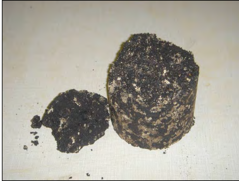
Figure 105. Failure of foamed asphalt stabilized sample during wet-dry testing
