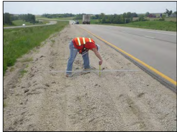
(b) Measuring rut depth inside the wheel path
