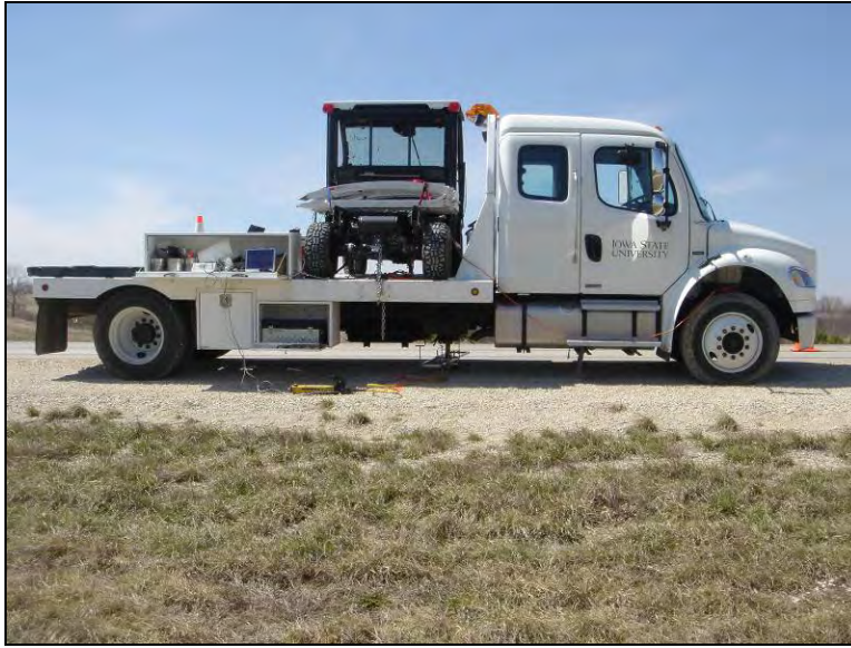
(a) Truck used as a reaction for performing the test
