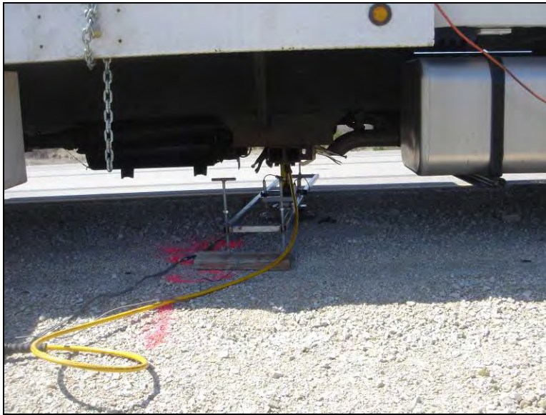
(b) Plate load test setup
