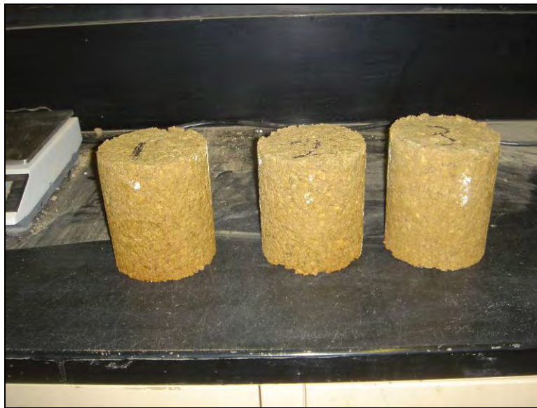
Figure 193. Soapstock-stabilized samples after vacuum saturation test
